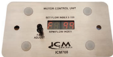
Figure 23. ECM control board – Non-modulating control with Trane unit controller (excludes Tracer® UC210 and UC400) or non-Trane unit controller
