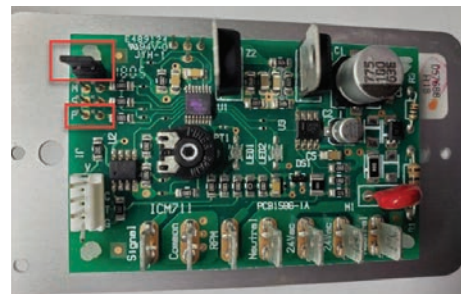
Figure 25. ECM control board 2-10 VDC input signal shunt placement
