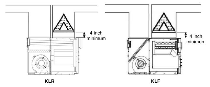
See A/C coil Manufacturers Requirements. To check the AC coil total air flow resistance, see procedure at page 38.
