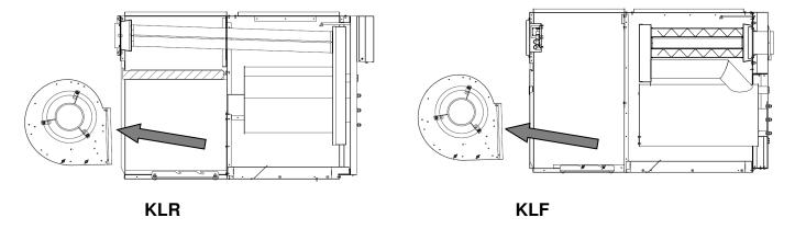
Put back the blower assembly using the reverse procedure. Ensure wiring and ground wires are correctly reconnected.
