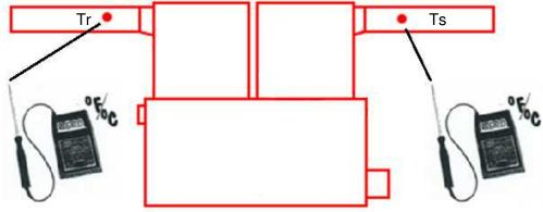
\*\*\* Probe must not be in direct sight of heat exchanger.
