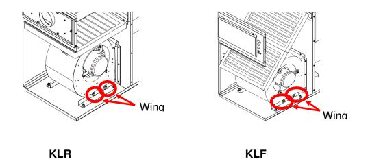
6) Slide the blower toward you and then lift the blower straight up. Shift the blower out of the furnace.
