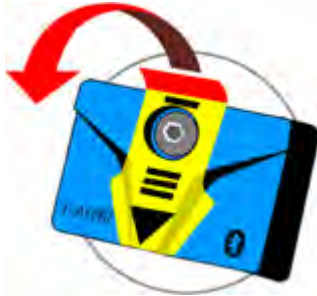
Figure 10: i-ALERT ® 2 Equipment Health Monitor activation
