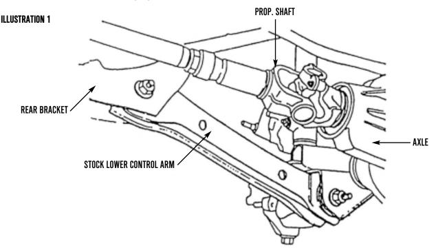
3) Disconnect the stock lower control arm at the axle and the rear bracket and remove. Refer to **ILLUSTRATION 2**.
