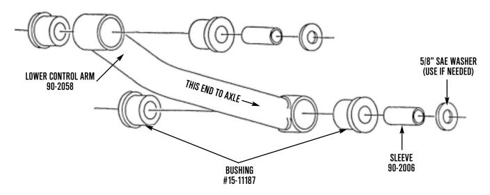
4) Position the lower control arms in the front and rear brackets and install using the existing bolts and nuts and the supplied washers if needed. See **ILLUSTRATION 3** and **4**.
