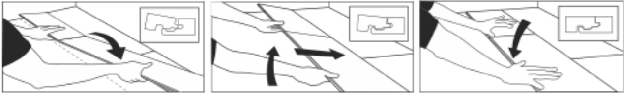
Fig. 5 Installing the second row.
