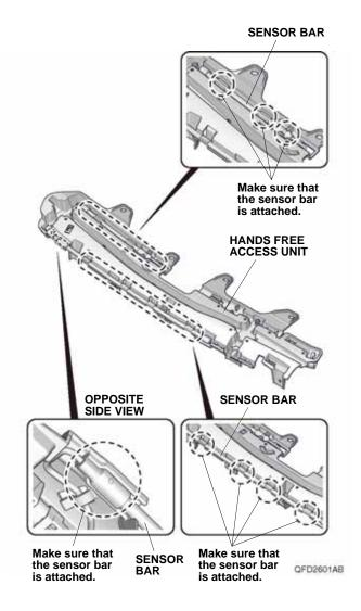
42. Install the hands free access unit to the rear bumper with two self-tapping screws, four clips, and one bumper clip. Go to step 51.
