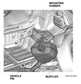
26. Remove the mounting rubber from the left side of the vehicle the same way, if equipped.
