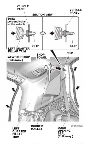
17. Using a rubber mallet wrapped with a shop towel, lightly tap the area marked "SIDE CURTAIN AIRBAG" on the left quarter pillar trim to push in the clip. Make sure to strike the area perpendicular to the vehicle.
