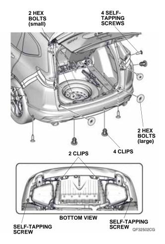
• With the help of an assistant, release the eight retaining tabs on each side.
