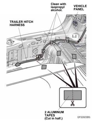
86. Using scissors, cut two aluminum tapes in half, and secure the trailer hitch harness to the vehicle panel with three halves of aluminum tape as shown.
