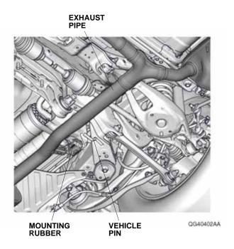
29. Using a utility knife, cut off the rear under cover as shown. Remove any burrs and sharp edges from the corners.
