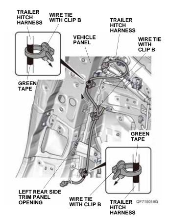
77. Secure the trailer hitch harness to the vehicle panel with one wire tie with clip B.
