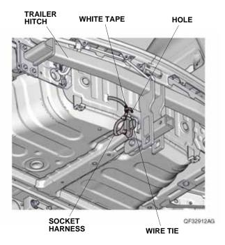
66. Remove the vehicle grommet. Route the socket harness through the vehicle panel hole.
