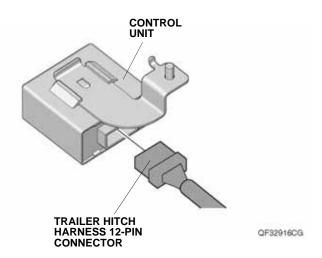
71. Install the control unit bracket to the vehicle panel with one 6 mm flange nut and one 6 mm plain washer.
