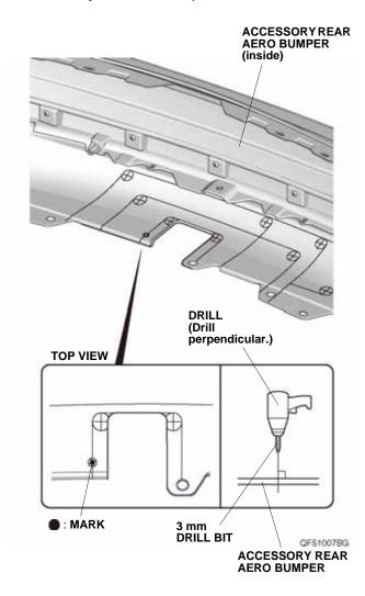
49. While wearing eye protection, enlarge the 3 mm hole to 14 mm using a 14 mm hole saw. Remove any burrs.
