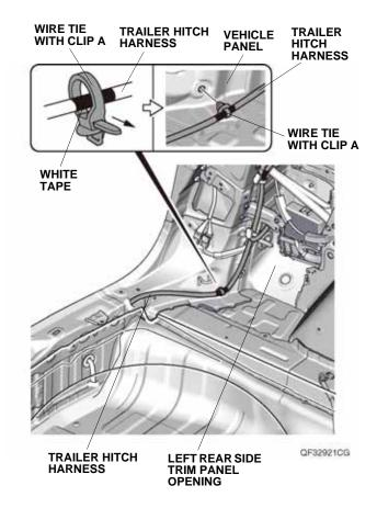
83. Peel back the floor carpet, then route the trailer hitch harness as shown.
