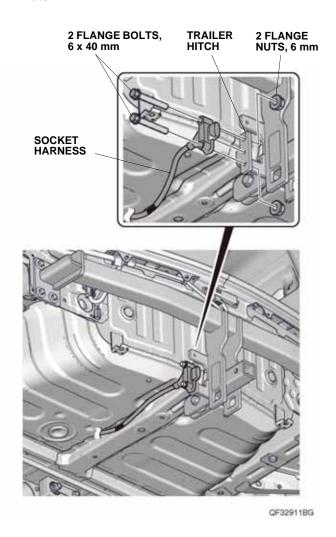
65. Line up the white tape on the socket harness to the hole on the trailer hitch, and secure the socket harness to the trailer hitch with one wire tie at the white tape on the socket harness.
