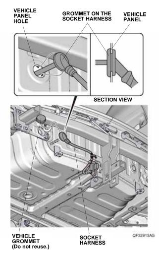
67. Install the grommet on the socket harness into the vehicle panel hole.
