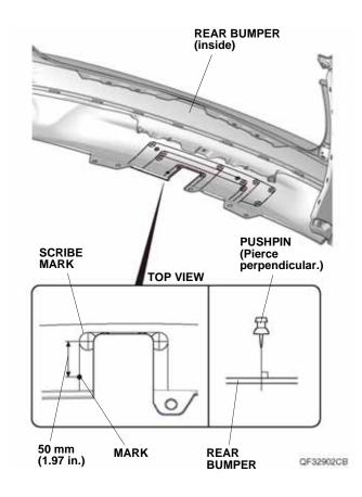
39. While wearing eye protection, drill the pierced mark on the rear bumper with a 3 mm drill bit. NOTE: Make sure to drill perpendicular to the rear bumper.
