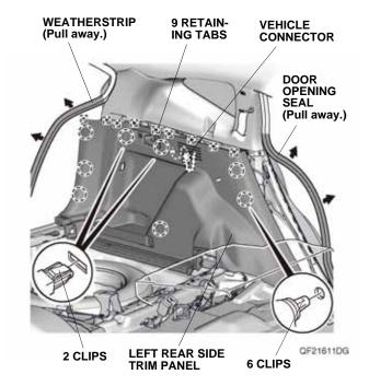
14. Release the cable from the left rear side trim panel, then remove the inner handle.
