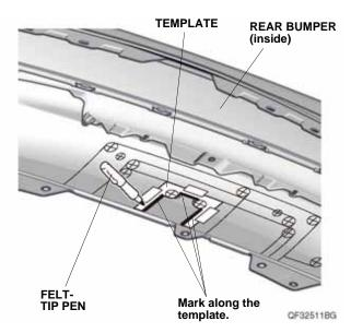
33. Using a pushpin, pierce two marks in the template on the rear bumper.
