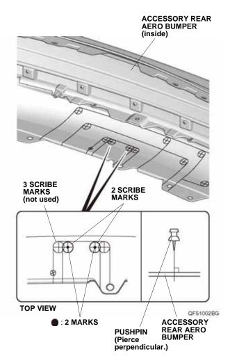
44. While wearing eye protection, drill the two pierced marks on the accessory rear aero bumper with a 3 mm drill bit.
