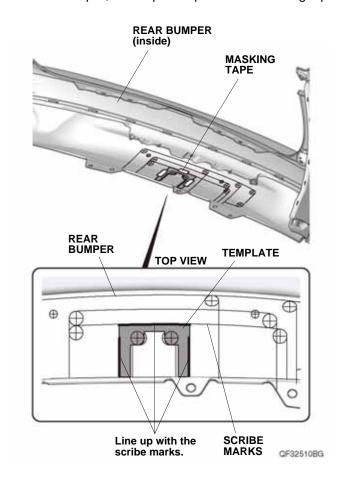
32. Using a felt-tip pen, mark the rear bumper along the template.
