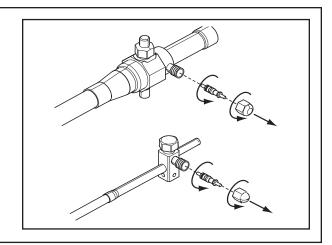
**STEP 3** - Purge the refrigerant lines and indoor coil with dry nitrogen.
