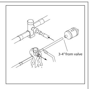
**STEP 5** - Replace the pressure tap valve cores after the service valves have cooled.
