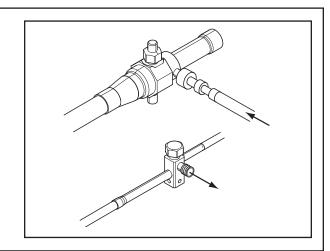
**STEP 4** - Wrap a wet rag around the valve body to avoid heat damage and continue the dry nitrogen purge.
