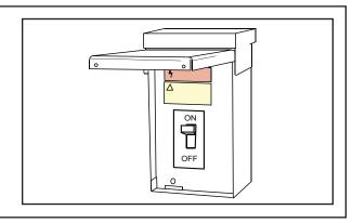
**STEP 4** - Wait one (1) hour before starting the unit if compressor crankcase heater accessory is used and the Outdoor Ambient is below 70°F.
