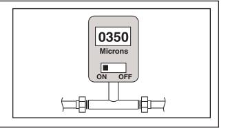
**STEP 2** - Observe the micron gauge. Evacuation is complete if the micron gauge does not rise above 500 microns in one (1) minute.
