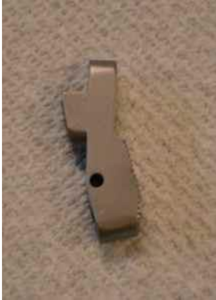
Bottom view of the bolt stop.
