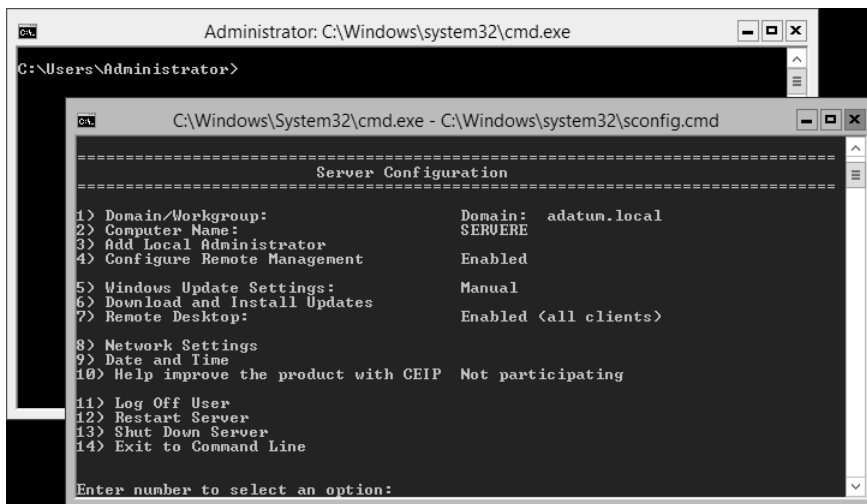
FIGURE 3-4 The Server Core interface in Hyper-V Server
