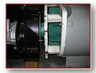
After the line-up studs are installed directly across from each other, level both the engine and the generator so they can come together without a bind.
