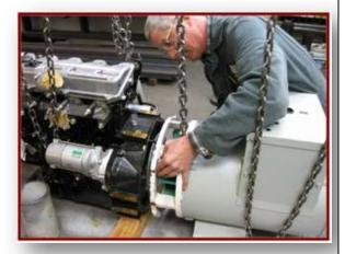
When the plates are bottomed put two bolts in the generator flange outer circle of bolts (only finger tight). Next remove the line-up studs and begin nstalling the drive plate bolts, again finger tight, one at a time, until they are all installed.
