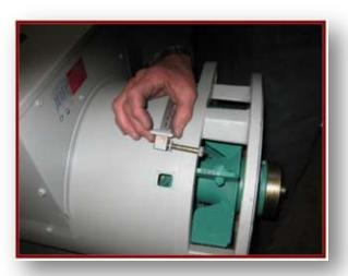
All it takes to bolt on the adapter is replacement of the dogs and their bolts after the new adapter is in place.
