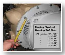
When drive plates require a change, the front housing adapter on the generator will, most often, need to be replaced as well.
