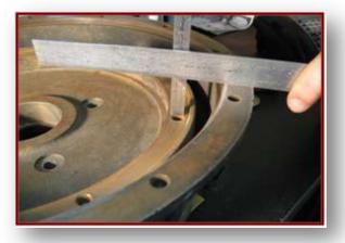
Be sure to verify that the flywheel and flywheel housing are the same SAE size as the drive face of the generator you are installing. To verify, measure the depth of the "g" dimension on the flywheel and the drive end of the generator.
