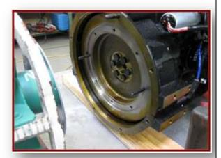
To insure a good fit to the engine, use a dial indicator and check the crankshaft thrust, which is also known as end-float. This is done with a dial indicator and is done before and after installing any crankshaft driven equipment (no matter if it is driven off the front or back end of the crankshaft). If this not done, the crankshaft may be forced hard against the crankshaft thrust bearing and it will cause the engine to fail.
