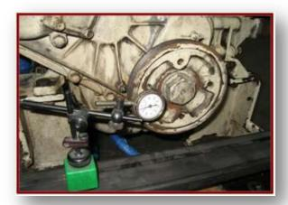
If the crank thrust is within manufacturers specifications, then proceed by inserting two line-up studs in the flywheel.
