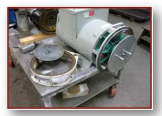
Every generator maker has a method for attaching the front adapter to the generator. In the case of this Marathon unit, there is a clever system of dogs that allow quick adapter change.
