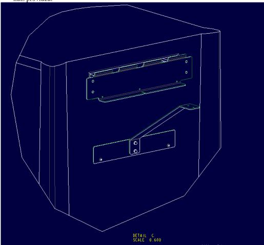
7. Remove the acorn nut from the bottom of the shelf that is closest to the side where the shelf frame mounts to the shelf rail, as shown in the following figure. (IMAGE FROM PREV. GUIDE)
