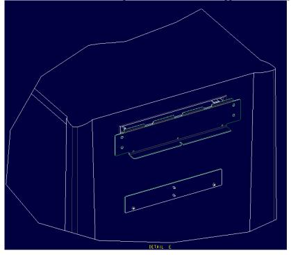
6. Place the Support Bracket on the Lower Brace as shown and secure in place with the two acorn nuts provided.
