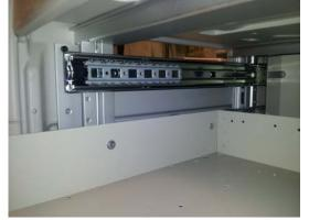
3. Slide the upper rail into the Artromick Cart's accessory slot until the upper rail is adjacent to the Artromick Cart Skin. Note the position of the two set screws located on the bare metal brackets, and adjust the two set screws if they are stopping the upper rail from sliding into place.
