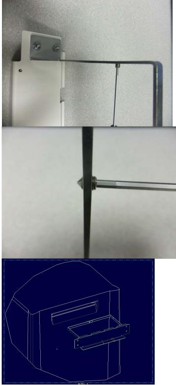
4. With a 3/32" Hex Socket driver, torque the previously removed set screws back into place to the depth shown in the figure. The bare metal bent metal brackets will bow when installing the set screws.
