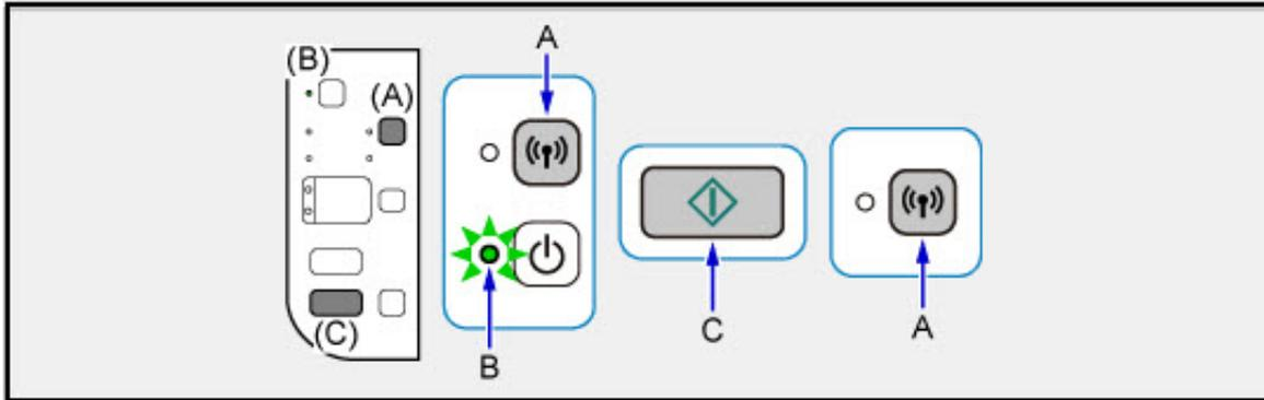
1. Hold down the **Wi-Fi button** (A) on the printer until the **ON lamp** (B) flashes, then release the **Wi-Fi button**.
