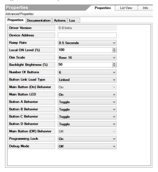
The first settings are identical to our Dimmer Driver. Here the added settings for Keypads:
