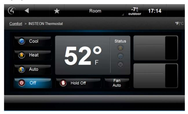
The INSTEON Thermostat driver is presented as a Control4 Wireless Thermostat in Navigator
