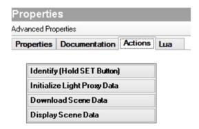
"Download Scene Data" will download all the link database from the dimmer and will save the final scene level of every scenes this dimmer is part of. The primary use of this action is to provide level feedback for this load in Navigator when a scene is triggered where it is part of. This process will generate LOT of INSTEON traffic and will complete only if there is no other traffic on the line. You can monitor the progress of the download on the Lua tab, it will show the
