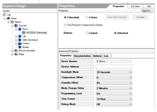
Most of these settings will auto-populate reflecting the actual configuration of the connected thermostat. If it does not, it may have a problem with the thermostat links, see troubleshooting section.
