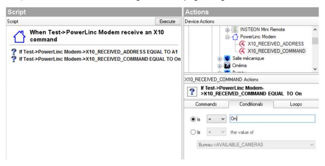
The X10\_RECEIVED\_ADDRESS will contain the X10 Address of the last X10 command received. The X10\_RECEIVED\_COMMAND will contact the last X10 command received.
