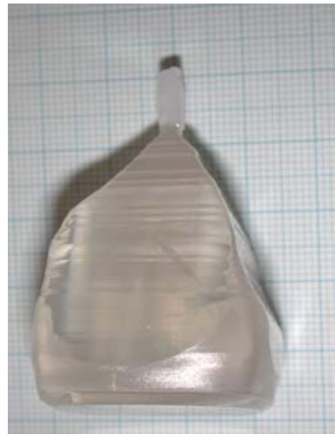
Undoped \text{KNbO}_3 crystal grown from [010]_c -oriented seed.
