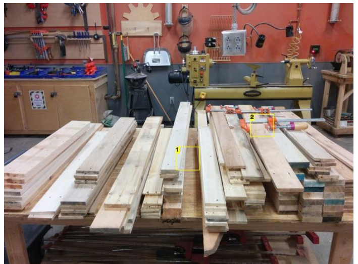
Image Notes 1. Consistent stock 2. Several pieces split in the process of cleaning; they were fixed using glue and clamps.
