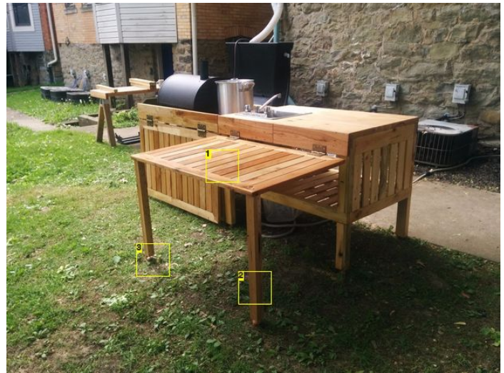
Image Notes 1. Fold-out table made from hardwood pallets 2. The table top can be removed and two additional legs added to have seating for 6-10 3. Leveling feet added to the table legs and uprights
