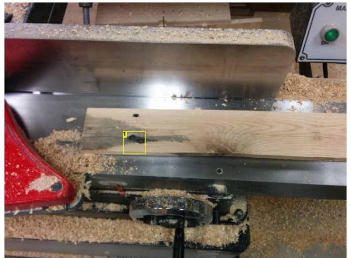
Image Notes 1. After - not necessary to remove everything, just to create a flat surface for the planer
