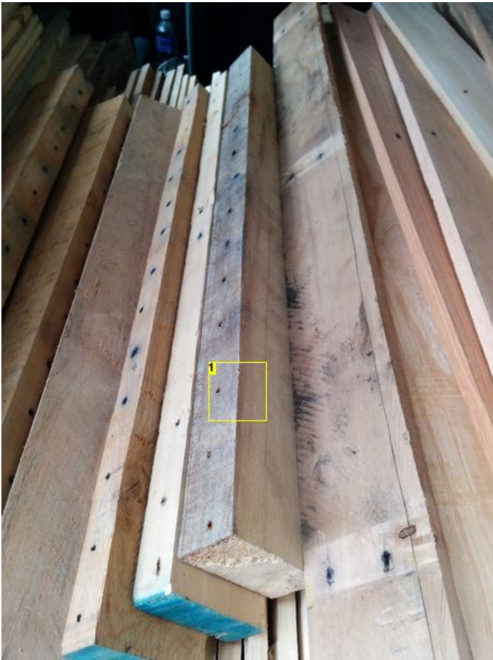
Image Notes 1. Pallet wood with nails removed, ready to be turned into consistent stock.
