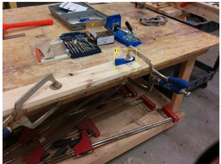
Image Notes 1. Drilling pocket holes in side spans and shelf supports
