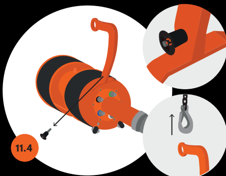
11.4 Disconnect the hoist from the weld isolation tool's hoisting hook
