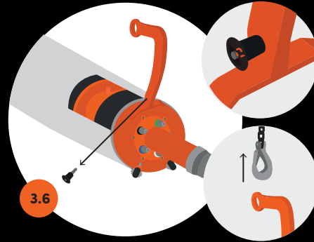
3.6 Disconnect the hoist from the weld isolation tool's hoisting hook
