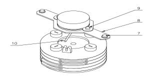
Turn the button P1 to operate the actuator in a closed or open direction. Put the actuator in open position. Using a screw rotate the came to the position in which it can trip the limit switch. Proceed the same way for the closed position. Put the power supply "OFF". Fix the potentiometer plate (item 8) and put the power supply "ON".
