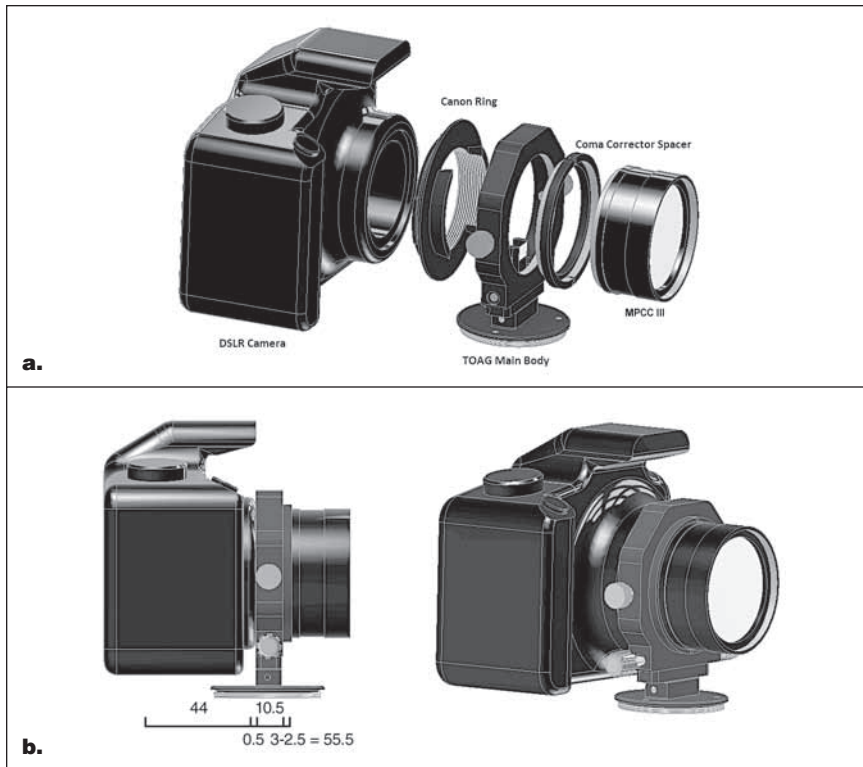
Figure 6. a) DSLR Camera with TOAG and MPCC spacer, b) Coma-corrector at the required distance to the camera sensor.
