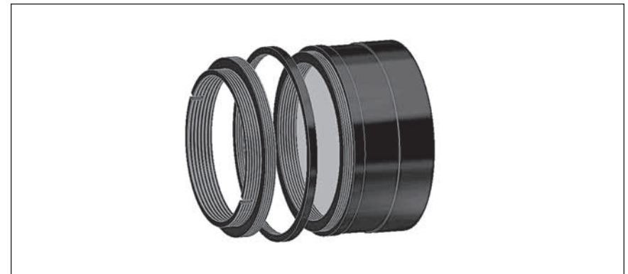
Figure 7. Removing the MPCC III T-threads adapter to expose the M48 threads.
