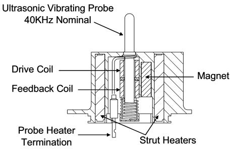
**Figure 1 MSO Circuit Sectional View**
