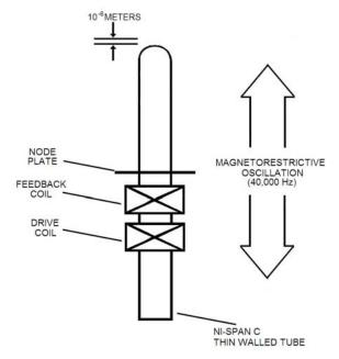
**Figure 2 MSO Circuit Schematic**
