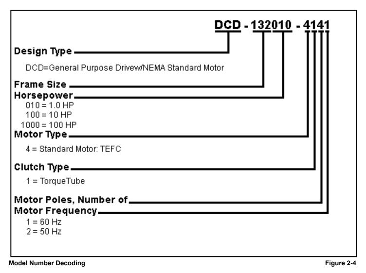
Models DCD-132 through DCD-225 Drive Ratings The basic Model DCD drive includes a TEFC AC induction motor flange mounted to an eddy-current clutch. Table 2-1 lists units requiring a 230/460 VAC, 3 phase, <u>60 Hz</u>, 1.15 SF input. NEMA design B, Class F insulation is used in all motors.
