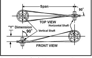
Perpendicular Shaft Alignment Figure 3-5
