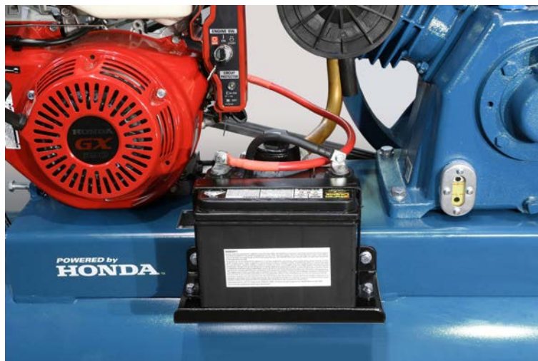
Figure 5-8 Puma 12 Volt Battery Kit Installed
