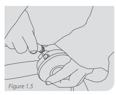
Connect the PTT cable to the head set cable and place the cable underneath the cape.
