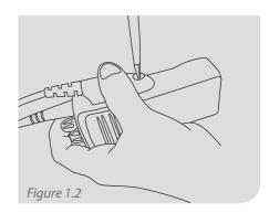
Use a Flat head screwdriver to tighten the connection screw.
