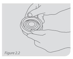
To fit, press the Protective Shroud onto the PTT.
