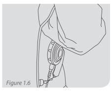
To operate the device, press your elbow onto the PTT Button, and then speak.
