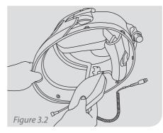
Place the Nova 3 Talk Sidepad into the helmet, ensuring that it is securely attached to the joining bracket.
