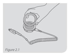
The Protective Shroud is used when working in positions that the PTT could be activated accidently.
