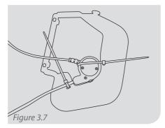
Place the headset on the right hand frame, and attach with cable ties as shown, then trim the ends of the cable ties.
