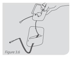
Remove the headset from the sidepad and cut the cable ties.
