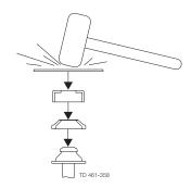
Study the instructions carefully. The items refer to the parts list and service kits section. Handle scrap correctly. A/A = Air/air activated.Service tool: See Spare Parts.
