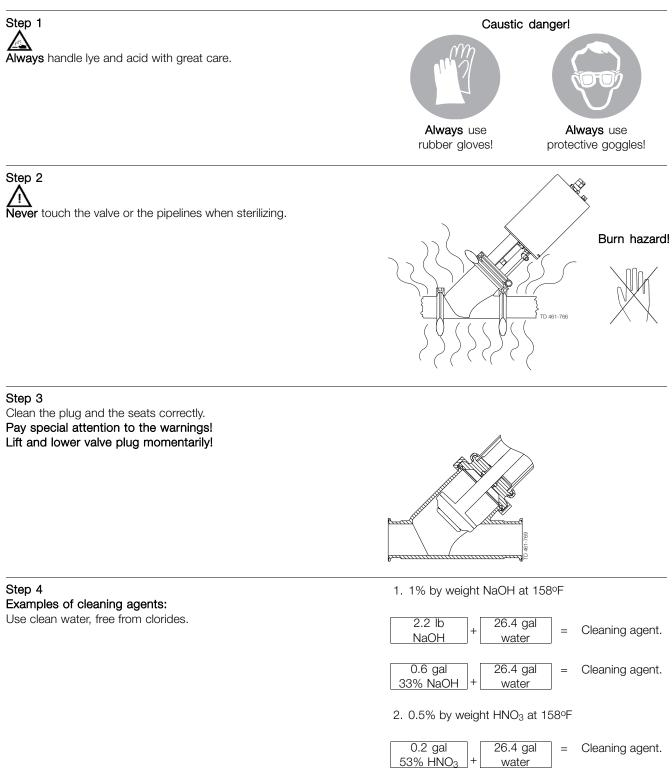
The valve is designed for cleaning in place (CIP). CIP = Cleaning In Place. Study the instructions carefully and pay special attention to the warnings! NaOH = Caustic Soda. HNO<sub>3</sub> = Nitric acid.
