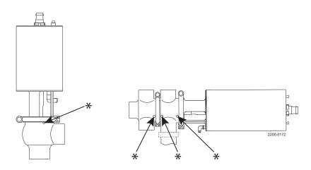
\* = Leakage detection hole
