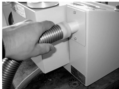
Insert dust aspirator hose on back connector
