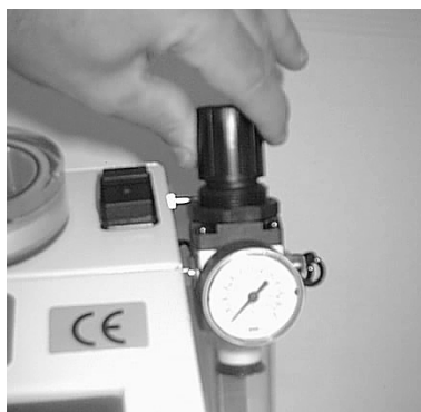
Regulate air pressure (min 2 – max 6 bars)
