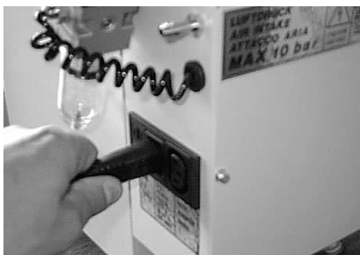
Connect aspirator plug in the sandblaster socket
