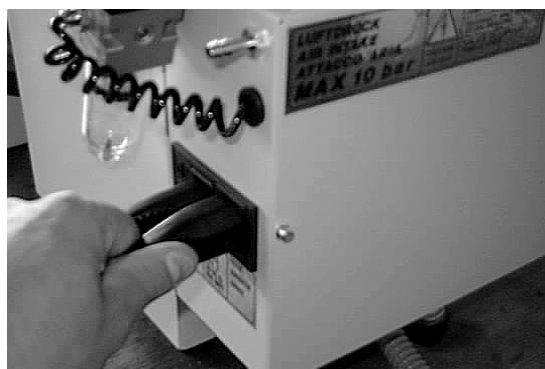
Insert plug respecting voltage on back plate
