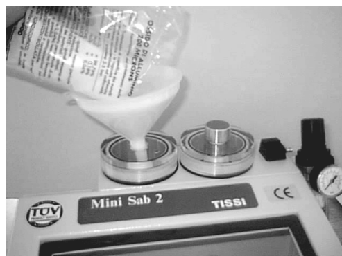
Fill containers with appropriate grain size of sand
