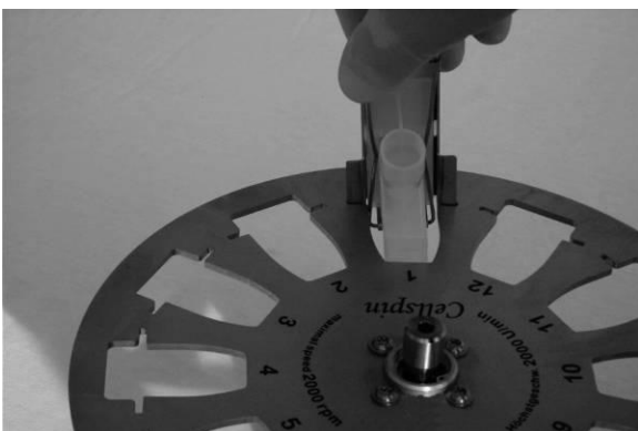
5. Insert the preparation system in the CellClip-rotor of the Cellspin® Cytocentrifuge.
