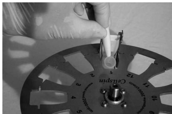
6. Shake vial with cell suspension and determine the turbidity. Depending on turbidity pipette 1-2 ml cell suspension into the ECOfunnel® .
