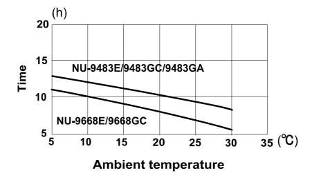
• The above data is the experiment value which uses liquid CO<sub>2</sub> 30L. (no-load)
