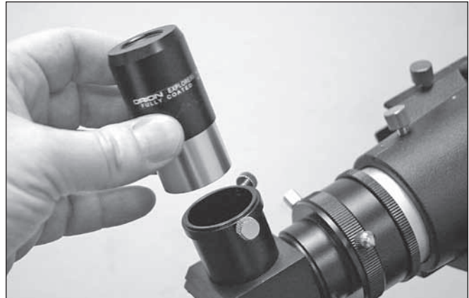
Figure 7. Insert the chrome barrel of the eyepiece into the diagonal and secure with the two thumbscrews. For the StarSeeker III reflector models, the eyepiece is inserted directly into the focuser's accessory adapter.
