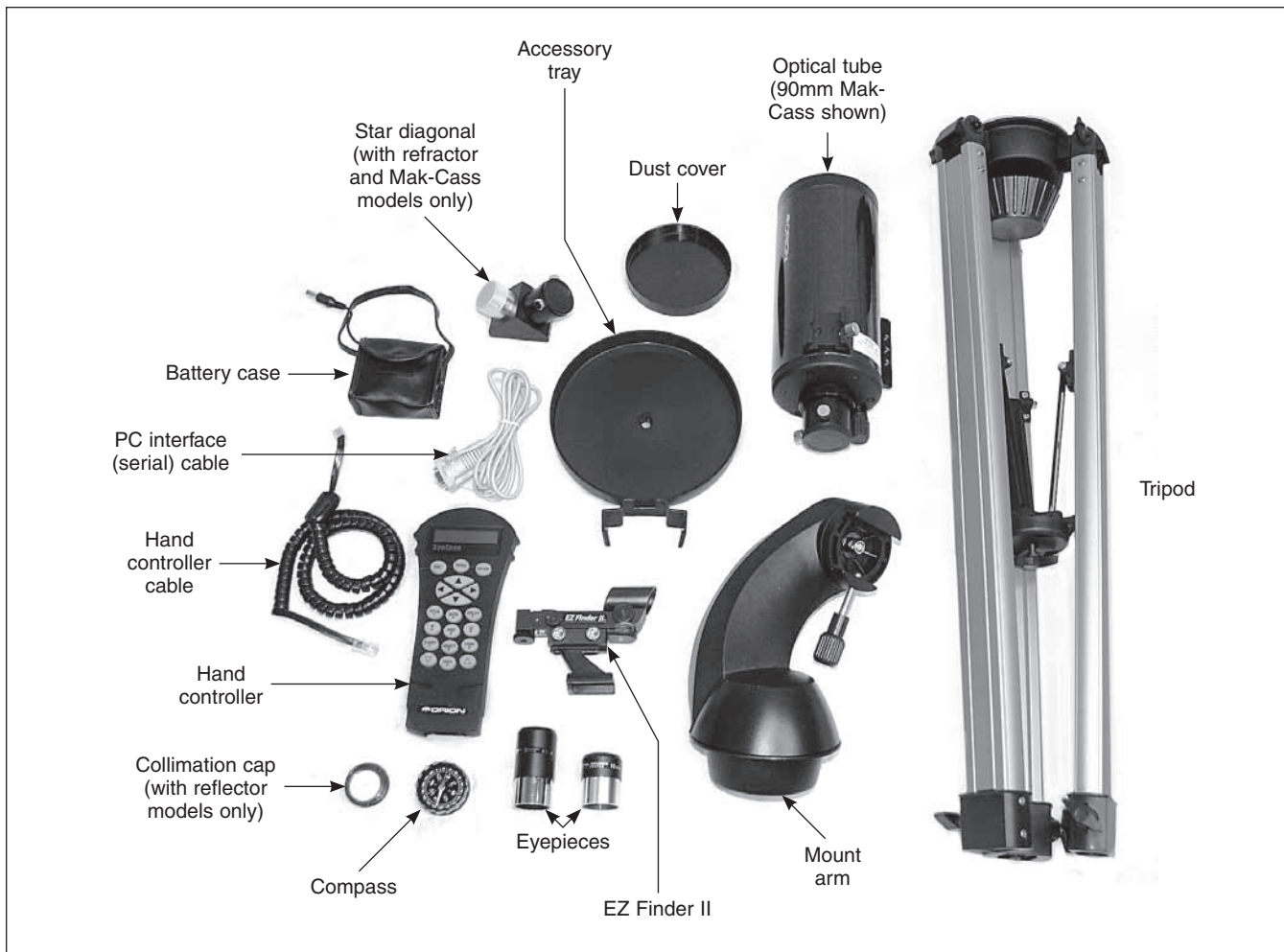
Figure 2. Components of the StarSeeker III GoTo telescope. (StarSeeker III 90mm Mak-Cass shown)
