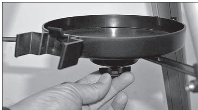
Figure 3. The round accessory tray attaches to the tripod leg brace with the captive screw on the brace.
