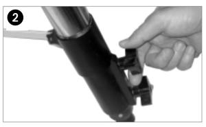
Thread in two lock-knobs on each leg (six total) near the foot of each tripod leg. Use the lockknobs to vary the height of the inner, extendible tripod leg sections. Tighten the locks to a firm feel only; do not overtighten.
