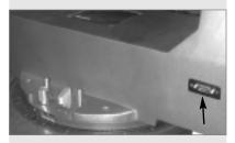
Fig. 52: DB-15 connector on fork base. Connect to the Dec motor port of the control panel.
