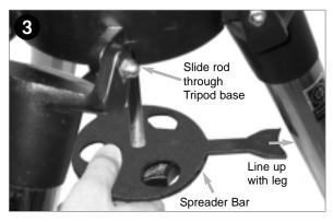
Remove the threaded rod from the tripod head. A small piece of plastic holds the threaded rod in place. Remove the small plastic bag that is stapled to the threaded rod. This bag contains the "C" clip retainer and an extra clip. Remove the spreader bar (see above figure) from the shipping carton. Slide the spreader bar onto the threaded rod. Slide the rod through the tripod base. Position the spreader bar so that its three arms line up with the three tripod legs.
