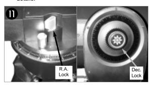
Tighten, to a firm feel only, the R.A. and Dec. locks. Remove the dust cover from the end of the telescope tube.
