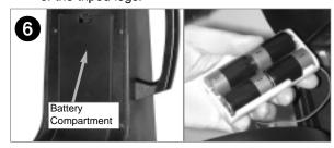
6. Remove the covers of the battery compartments located on the fork arms (one on each fork arm) and carefully lift the battery holders from their compartments, being mindful of the connector wires. Insert four (user-supplied) C-cell batteries into each battery holder, oriented as shown on the diagram on the battery holder. Return the battery holders to their respective compartments. Replace the covers when you are done.
