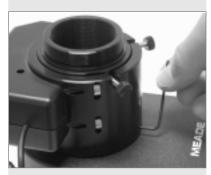
Fig. 56: Tighten the three microfocuser hex screws to a firm feel.
