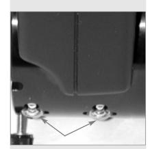
Fig. 30: Microfocuser ball bearings.
