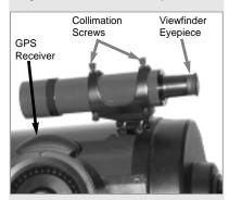
Fig. 12: Viewfinder collimation screws and eyepiece.
