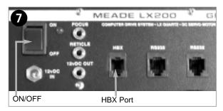
7. Press the computer control panel power switch to OFF, if necessary. Remove the Autostar II handbox and the Autostar II coil cord from the packing materials. Plug one end into the HBX port of the telescope's computer control panel and plug the other end into the coil cord port on the Autostar II handbox.
