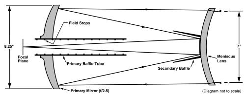
The Meade 7" Maksutov-Cassegrain design optimizes imaging performance by utilizing a combination of a two-sided spherical meniscus lens (right), a strongly aspheric f/2.5 primary mirror, and a spherical secondary mirror. The convex secondary mirror multiplies the effective focal length of the primary by a factor of six, resulting in an overall a focal length of 2670mm and a focal ratio of f/15 system at the Cassegrain focus.
