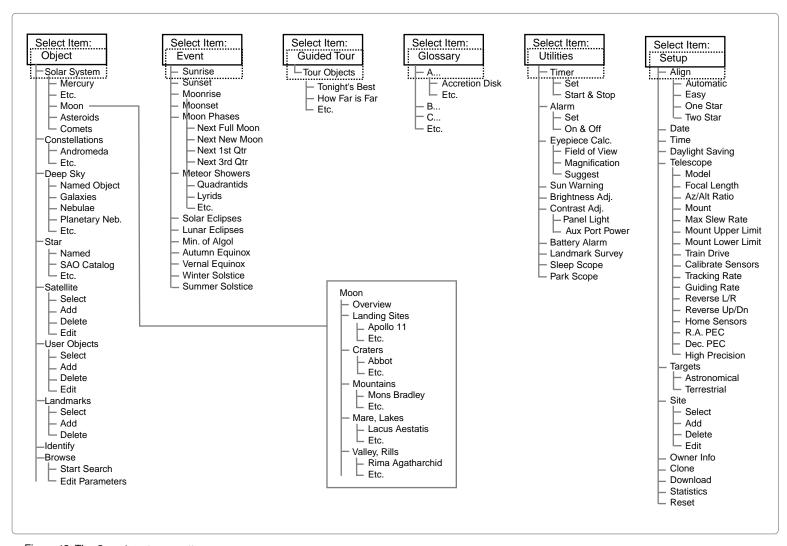
Figure 18: The Complete Autostar II Menu Tree Structure.
