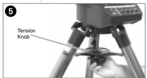
5. Take the LX200GPS from its packaging and place the entire telescope onto the top of the tripod head, inserting the threaded rod into the central hole in the bottom of the drive base of the telescope. Tighten the tension knob (see above figure) to a firm feel only; firm tightening of the tension knob is sufficient to result in rigid positioning of the tripod legs.
