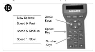
10. Press the key prompted by Autostar II to accept the Sun warning. Autostar II now attempts to gain a GPS fix; press any key to abort. Once aborted, keep pressing ENTER to bypass the Time, Date, and other menus until "Setup: Align" displays. You can then use the Arrow keys to slew (move) the telescope up, down, right, or left. To change the telescope's slew speed, press the Speed key and then the Number keys. "9" is the fastest speed and "1" is the slowest speed. See page 17 for more details.
