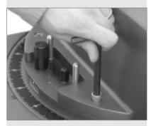
Fig. 49: Bolt the fork to the drive base.
