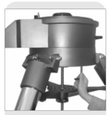
Fig. 48: Attach the drive base to the tripod.
