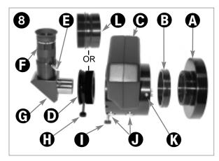
8. Attach microfocuser: Remove the dust cap from the rear cell port (A) of the telescope (Note: Telescope not shown for clarity). Thread the microfocuser adapter (B) into the rear cell port thread. Slide the microfocuser (C) over the microfocuser adapter and tighten the three hex screws on the microfocuser (K) using the provided hex keys.
