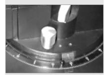
Fig. 36: Section of Right Ascension Setting Circle.
