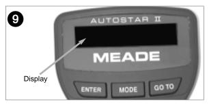
Press the Power Switch on the computer control panel to the ON position. The copyright message lights on Autostar II's LCD display.
