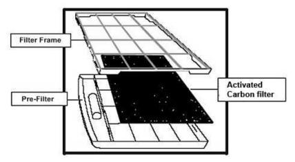
An optional 3M<sup>™</sup> Antimicrobial Filter can also be purchased to replace the activated carbon filter. The 3M<sup>™</sup> Antimicrobial Filter has an antimicrobial agent helps inhibit the growth of mold and mildew on the filter. This filter is electrostatically charged for enhanced particle capture and retention.
