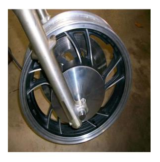
The RH end of the axle and/or the RH axle spacer may need to be modified as shown to tune-in the wheel/rotor centering position and allow the axle nut to be final torqued and cotter pinned. Carefully modify the axle as required.
