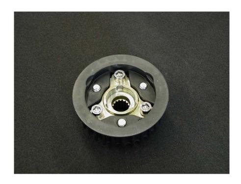
11. Re-install pulley to factory specs with new outer seal. (Don't forget to lube case seal before assembly).
