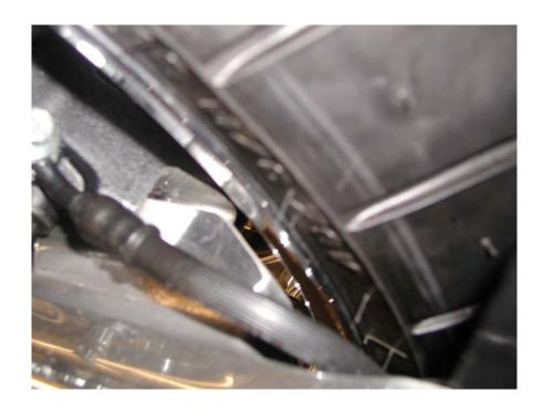
4. Clean up casting mark on inside of swingarm in pulley area (as pictured).
