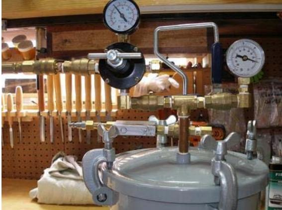
Air line connected and filling the tank with pressure,
