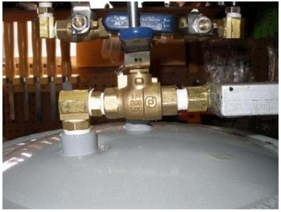
Come out of the vacuum block with your 1/4" air compressor fitting. The fittings that came mounted on the block work well for this. I tried to find a better method to attach the air compressor fitting, but the brass fitting that threads into that end of the block has a unique design which incorporates an "O" ring. The method I used was the best "I" could do with what I had available.
