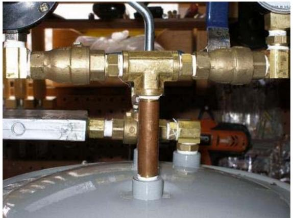
We will start at the air inlet of the tank. 1/4"x2 1/2" nipple in tank lids 1/4" opening, 1/4" "T", 1/4"x1" nipples in both sides of "T", 1/4" ball valves in both nipples (now both sides should look the same).
