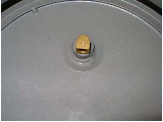
That's the extent of the assembly. Next you will want to do a pressure check. The first series of tests I ran where to simply fill the tank with air and let it sit. On the first test, I lost about 3 or 4 pounds of pressure in 24 hours. I did the soapy water test and found only one leak. It was at the cap on the side of the regulator.
