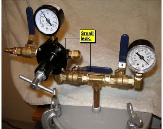
This was easily fixed with by re-taping the fitting and threading it back on. Now I have no noticeable leaks in the system.
