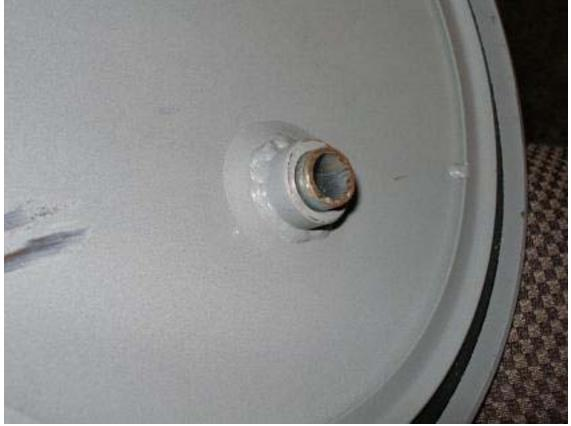
Once the lid was stripped down, it was time to begin the assembly process. Be sure and have lots of Teflon tape handy. I wrapped each fitting 5 to 7 times to insure each joint was sealed. Do not to get tape inside the ends of the fittings. You don't want it making its way into the pot or your vacuum pump. (Which really isn't a pump, I'll explain this more later)
