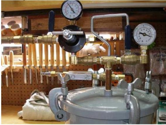
Tank full of pressure and air line shut off,
