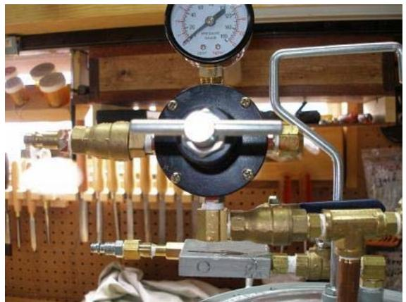
Now the left side, out of the ball valve, 1/4" elbow with female pointing up, pressure regulator in elbow facing you, 1/4" female cap in right side, 1/4" ball valve in left side, 1/4" air compressor fitting
