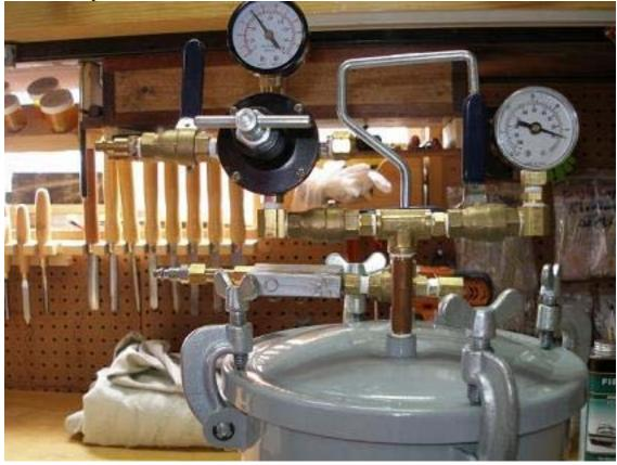
Tank full of pressure and line removed,
