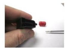
STEP 41F: Insert the terminal (from STEP 41D) into the NEW replacement connector, noting the orientation of the terminal. A locating tab on the terminal will allow the terminal to insert in only one direction.
