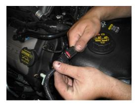
STEP 43: Clip the remaining (2) connectors on the jumper harness to the throttle body.
