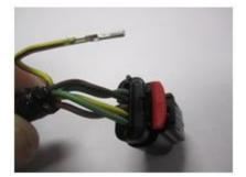
**STEP 41E:** Prepare the NEW replacement connector for terminal insertion by removing the red retaining lock from the connector. Like the previous connector, this lock can also be removed by gently prying out.
