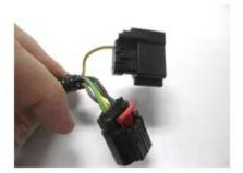
STEP 41G: Return to STEP 41C, and follow the same sequence for Pin 2 through Pin 6. Once all six terminals have been moved, replace the red locking tab (previously referred to in STEP 41E).
