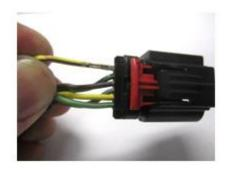
**STEP 41D:** Completely remove the wire and terminal from the factory connector.
