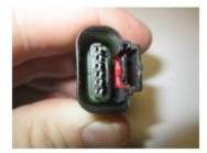
Starting with Pin 1, carefully pry back the plastic retaining tab (which holds the female terminal into the connector housing) while gently pulling on the wire from behind until the terminal has been released.
