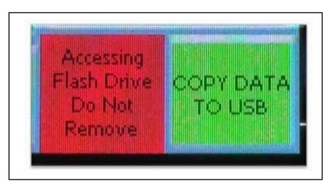
Figure 6: Copy Data to USB Button and Red "Accessing USB Drive Do Not Remove" Alert
