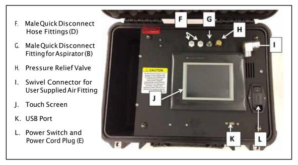
Figure 2: Test Kit Layout
