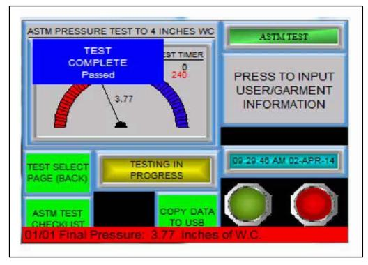
Figure 11: End of Test Output Display
