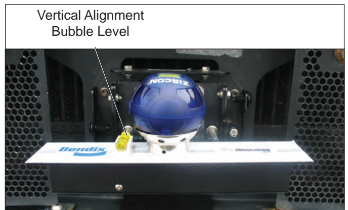
FIGURE 30 - VERTICAL ALIGNMENT BUBBLE LEVEL
