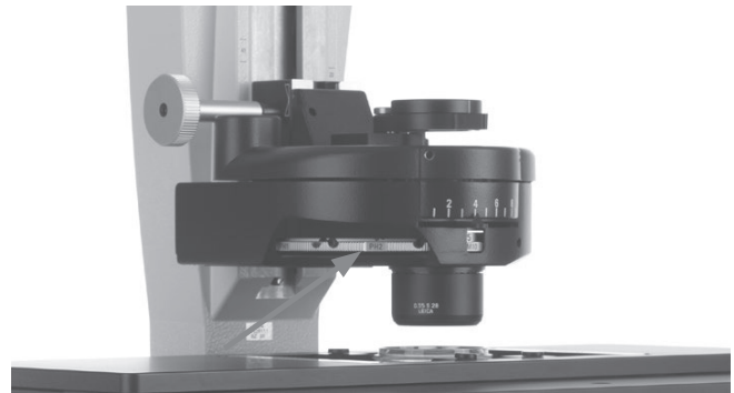
Condenser setting for tiltable Transmitted Light arm - configuring Darkfield stop (light ring)
