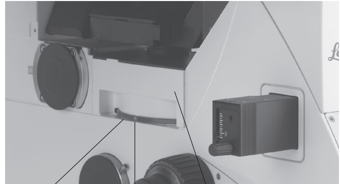
Color mark Knurled ring for setting the filter cube Cover
