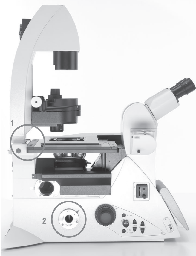
Interlock switch (1) and (2)
