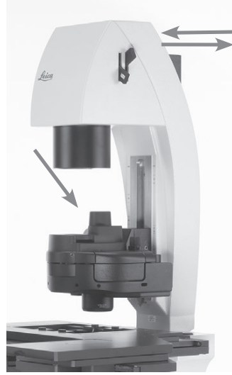
Folded back Transmitted Light arm; the light output out of the objective is not shadowed by the condenser base.
