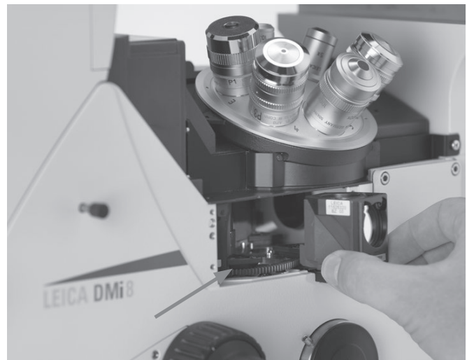
Empty position for mounting a filter cube. The filter cube is pushed in from the front evenly until it clicks into place.
