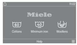
Up to 12 pre-set programmes are available. The first 3 programmes can be selected directly. The remaining programmes are selected from a list \(\mathbb{H}\). These cannot be changed by the operator.
