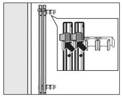
Secure the transit bars to the back of the washing machine. Make sure that the top catch is located above the holder.
