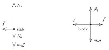
Applying Newton's second law for the x and y axes for (first) the slab and (second) the block results in four equations:
