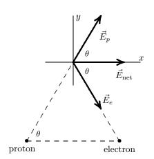
$$\begin{aligned} \left| \vec{E}_{\text{net}} \right| &= E_x = 2E_e \cos \theta \\ &= 2\left(\frac{e}{4\pi\varepsilon_0 d^2}\right) \cos \theta = 2k \left[\frac{e}{d^2}\right] \cos \theta \\ &= 2\left(8.99 \times 10^9 \,\frac{\text{N} \cdot \text{m}^2}{\text{C}^2}\right) \left[\frac{(1.6 \times 10^{-19} \,\text{C})}{(2.0 \times 10^{-6} \,\text{m})^2}\right] \cos 60^\circ \\ &= 3.6 \times 10^2 \,\text{N/C} \,. \end{aligned}$$
