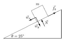
(a) With the x axis directed up along the incline (so that  $a = -0.86 \text{ m/s}^2$ ), Newton's second law leads to
