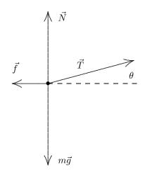
(b) The second law equations for the moving crate are  $T \cos \theta - f = ma$  and  $N + T \sin \theta - mg = 0$ . Now  $f = \mu_k N$ . The second equation gives  $N = mg - T \sin \theta$ , as before, so  $f = \mu_k (mg - T \sin \theta)$ . This expression is substituted for f in the first equation to obtain  $T \cos \theta - \mu_k (mg - T \sin \theta) = ma$ , so the acceleration is
