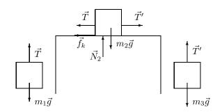
We use the familiar axes with +x rightward and +y upward for each block. This has the consequence that  $m_1$  and  $m_2$  accelerate with the same sign, but the acceleration of  $m_3$  has the opposite sign. We take this into account as we apply Newton's second law to the three blocks.
