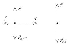
(b) The second law equations become  $T - f = (W_A/g)a$ ,  $N - W_A = 0$ , and  $W_B - T = (W_B/g)a$ . In addition,  $f = \mu_k N$ . The second equation gives  $N = W_A$ , so  $f = \mu_k W_A$ . The third gives  $T = W_B - (W_B/g)a$ . Substituting these two expressions into the first equation, we obtain  $W_B - (W_B/g)a - \mu_k W_A = (W_A/g)a$ . Therefore,
