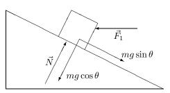
(a) The trunk is moving up the incline at constant velocity, so a = 0. Using  $f_k = \mu_k N$ , we solve for the push-force  $F_1$  and obtain
