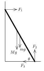
(a) Since the ladder is in equilibrium the sum of the torques about its foot (or any other point) vanishes. Let  $\ell$  be the distance from the foot of the ladder to the position of the window cleaner. Then,  $Mg\ell\cos\theta + mg(L/2)\cos\theta - F_1L\sin\theta = 0$ , and
