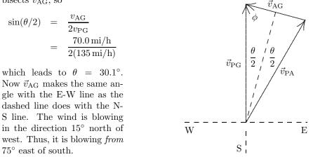
(b) The plane is headed along  $\vec{v}_{PA}$ , in the direction  $30^{\circ}$  east of north. There is another solution, with the plane headed  $30^{\circ}$  west of north and the wind blowing  $15^{\circ}$  north of east (that is, from  $75^{\circ}$  west of south).
