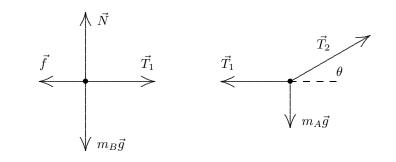
For each object we take +x horizontally rightward and +y upward. Applying Newton's second law in the x and y directions for block B and then doing the same for the knot results in four equations:
