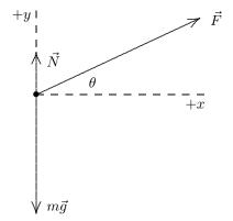
(b) If F is the minimum force for which the block leaves the floor, then N = 0 and the y component of the acceleration vanishes. The y component of the second law becomes  $F \sin \theta - mg = 0$ , so
