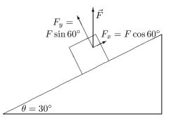
(a) Assuming the block is not pulled entirely off the incline, Newton's second law applied to the x axis yields
