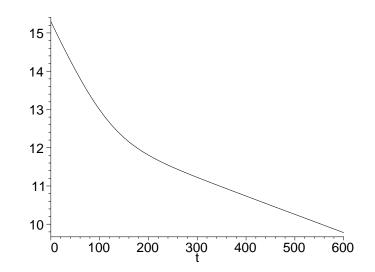
We note that the magnitude of the slope for small t is  $\lambda'$  (the disintegration constant for <sup>110</sup>Ag), and for large t is  $\lambda$  (the disintegration constant for <sup>108</sup>Ag).
