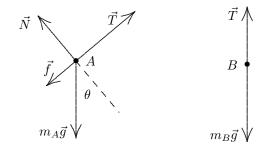
Since A is moving down the incline, the force of friction is uphill with magnitude  $f_k = \mu_k N$  (where  $\mu_k = 0.20$ ). Newton's second law leads to
