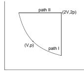
(b) "Path I" consists of an isothermal (constant T) process in which the volume doubles, followed by a constant-volume process. We consider the Q for each of these steps. We note that the connection between molar heat capacity and the degrees of freedom of a monatomic gas is given by setting f = 3 in Eq. 20-51. Thus,  $C_V = \frac{3}{2}R$ ,  $C_p = \frac{5}{2}R$ , and  $\gamma = \frac{5}{3}$ .
