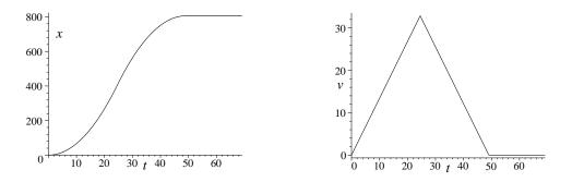
80. Average speed, as opposed to average velocity, relates to the total distance, as opposed to the net displacement. The distance D up the hill is, of course, the same as the distance down the hill, and since the speed is constant (during each stage of the motion) we have speed = D/t. Thus, the average speed is
