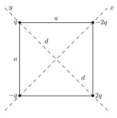
At the center of the square, the field produced by the charges at the upper left and lower right corners are both along the y axis and each points away from the charge that produces it. The net field produced at the center by these charges is
