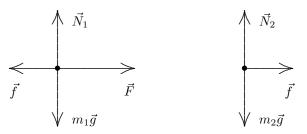
(a) Newton's second law for block 1 is  $F - f = m_1 a$ , where a is the acceleration. The second law for block 2 is  $f = m_2 a$ . Since the blocks move together they have the same acceleration and the same symbol is used in both equations. From the second equation we obtain the expression  $a = f/m_2$ , which we substitute into the first equation to get  $F - f = m_1 f/m_2$ . Therefore,
