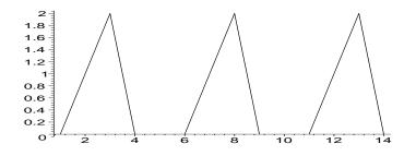
(d) The leading edge of the pulse reaches x = 10 cm at t = (10 - 4)/5 = 1.2 s. The particle (say, of the string that carries the pulse) at that location reaches a maximum displacement h = 2 cm at t = (10 - 3)/5 = 1.4 s. Finally, the the trailing edge of the pulse departs from x = 10 cm at t = (10 - 1)/5 = 1.8 s. Thus, we find for h(t) at x = 10 cm (with the horizontal axis, t, in seconds):
