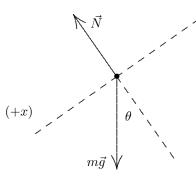
(a) Placing the origin at the bottom of the plane, the kinematic equations (Table 2-1) for motion along the x axis which we will use are  $v^2 = v_0^2 + 2ax$  and  $v = v_0 + at$ . The block momentarily stops at its highest point, where v = 0; according to the second equation, this occurs at time  $t = -v_0/a$ . The position where it stops is
