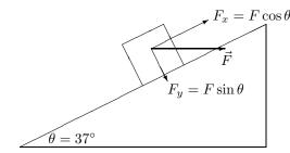
(a) Applying Newton's second law to the x (directed uphill) and y (directed away from the incline surface) axes, we obtain
