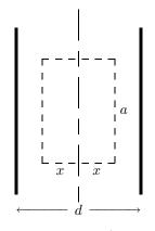
The volume enclosed by the Gaussian surface is  $2a^2x$  and the charge contained within it is  $q = 2a^2x\rho$ . Gauss' law yields  $2\varepsilon_0 Ea^2 = 2a^2x\rho$ . We solve for the magnitude of the electric field:
