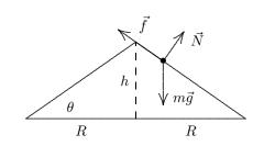
Since R and h are two sides of a right triangle,  $h = R \tan \theta$ . Replacing  $\tan \theta$  with  $\mu_s$  we obtain  $h = \mu_s R$ . We substitute this into the volume equation  $V = \pi R^2 h/3$  to obtain the result  $V = \pi \mu_s R^3/3$ .
