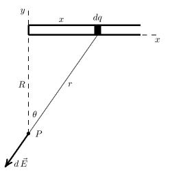
We use  $\theta$  as the variable of integration and substitute  $r = R/\cos\theta$ ,  $x = R\tan\theta$  and  $dx = (R/\cos^2\theta) d\theta$ . The limits of integration are 0 and  $\pi/2$  rad. Thus,
