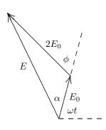
Here d is the center-to-center slit separation and  $\lambda$  is the wavelength. The resultant wave can be written  $E = E_1 + E_2 = E \sin(\omega t + \alpha)$ , where  $\alpha$  is a phase constant. The phasor diagram is shown above. The resultant amplitude E is given by the trigonometric law of cosines:
