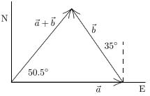
(a) Let  $\vec{c} = \vec{a} + \vec{b}$ . Then  $c_x = a_x + b_x = 5.0 \text{ m} - 2.29 \text{ m} = 2.71 \text{ m}$  and  $c_y = a_y + b_y = 0 + 3.28 \text{ m} = 3.28 \text{ m}$ . The magnitude of c is
