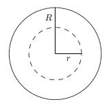
If  $\rho$  is positive, the electric field lines are radially outward, normal to the Gaussian surface and distributed uniformly along it. Thus, the total flux through the Gaussian cylinder is  $\Phi = EA_{\text{cylinder}} = E(2\pi r\ell)$ . Now, Gauss' law leads to
