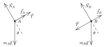
For each block we take +x downhill (which is toward the lower-left in these diagrams) and +y in the direction of the normal force. Applying Newton's second law to the x and y directions of first block A and next block B, we arrive at four equations:
