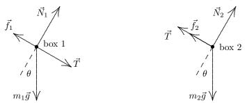
For each block we take +x downhill (which is toward the lower-right in these diagrams) and +y in the direction of the normal force. Applying Newton's second law to the x and y directions of first box 2 and next box 1, we arrive at four equations:
