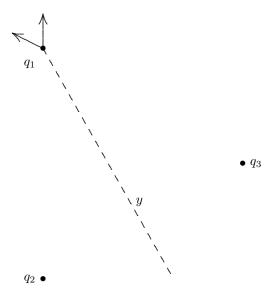
The y axis is meant to bisect the line between  $q_2$  and  $q_3$  in order to make use of the symmetry in the problem (equilateral triangle of side length d, equal-magnitude charges  $q_1 = q_2 = q_3 = q$ ). We see that the resultant force is along this symmetry axis, and we obtain
