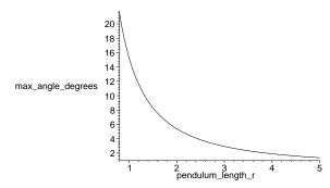
(h) The original value of  $\theta_{\text{max}}$  is  $\cos^{-1}(1 - 0.0353/r_0^3)$  where  $r_0 = 0.80$  m. This gives 21.4° as the initial "turning point" angle. The question, then, asks us to solve for r in the case that  $\theta_{\text{max}} = \frac{1}{2}(21.4^\circ) = 10.7^\circ$ . We know to look for half the initial value (as opposed to one twice as big) because the previous part shows  $\theta_{\text{max}}$  decreases with r. This value of the turning point angle occurs for
