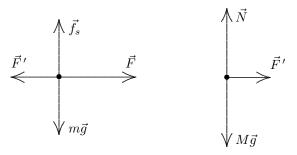
Treating the two blocks together as a single system (sliding across a frictionless floor), we apply Newton's second law (with +x rightward) to find an expression for the acceleration.
