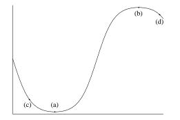
Any change from zero to non-zero values of  $\vec{v}$  represents increasing  $|\vec{v}|$  (speed). Also,  $\vec{v} \parallel \vec{a}$  implies that the particle is going faster. Thus, points (a), (b) and (d) involve increasing speed.
