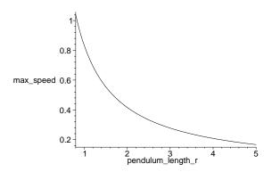
(n) When  $r = r_0$  we find  $v_{\text{max}} = 1.04$  m/s. Any later value must be smaller (according to the above graph), so we seek a value of r that gives  $v_{\text{max}} = 0.520$  m. This can be solved for algebraically:
