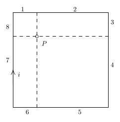
Let  $\vec{e}$  be a unit vector pointing into the page. We use the results of problems 13 and 16 to calculate  $B_{P1}$  through  $B_{P8}$ :
