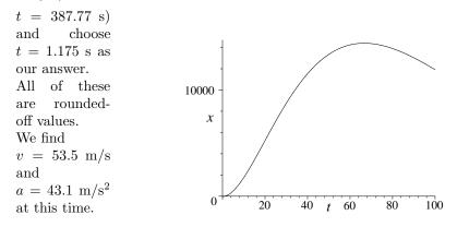
(d) It is much easier to find when  $24t(2 - 0.03t)e^{-0.03t} = 0$  since the roots are clearly  $t_1 = 0$  and  $t_2 = 2/0.03 = 66.7$  s. We find  $x(t_1) = -32.0$  m and  $a(t_1) = 48.0$  m/s<sup>2</sup> at the first root, and we find  $x(t_2) = 1.44 \times 10^4$  m and  $a(t_2) = -6.50$  m/s<sup>2</sup> at the second root.
