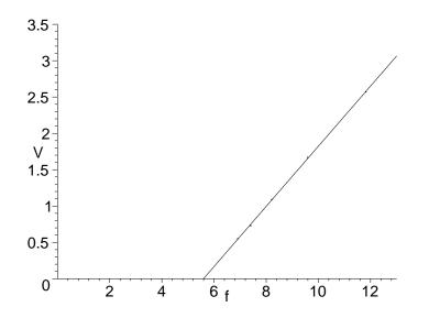
From our least squares fit procedure, we determine the slope to be  $4.14 \times 10^{-15}$  V·s, which is in very good agreement with the value given in Eq. 39-3 (once it has been multiplied by e).
