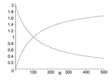
(c) In our final graph, we show the dependence of power  $P = iV_R$  (dissipated in resistor R) as a function of R. The units of the vertical axis are Watts. We note that it is maximum when R = r.
