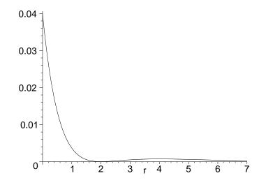
(b) The extrema of  $\psi^2(r)$  for  $0 < r < \infty$  may be found by squaring the given function, differentiating with respect to r, and setting the result equal to zero:
