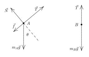
(a) For A we take the +x to be uphill and +y to be in the direction of the normal force. The x and y components of Newton's second law become
