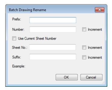
The user must enter a value into the **Number** field. The value can be numbers, letters or a combination of the two. If the user enters any letters the **Increment** checkbox next to the **Number** field cannot be used. If only numbers are entered, the user may check the **Increment** box. This causes the Drawing Numbers of the selected items to be incremented by one.
