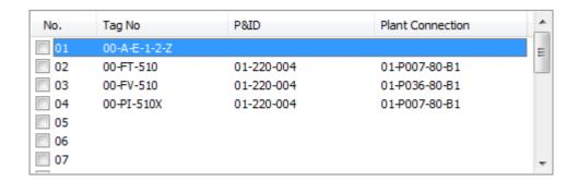
This will automatically move all tag data on the corresponding hookup drawing to the new positions next time the drawing is updated.
