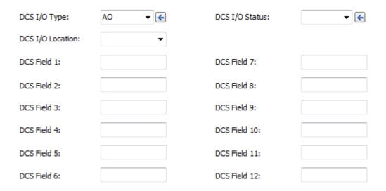
The DCS System tab is used to assign DCS I/O information for the current tag (if the current tag will be connected to the DCS System).
