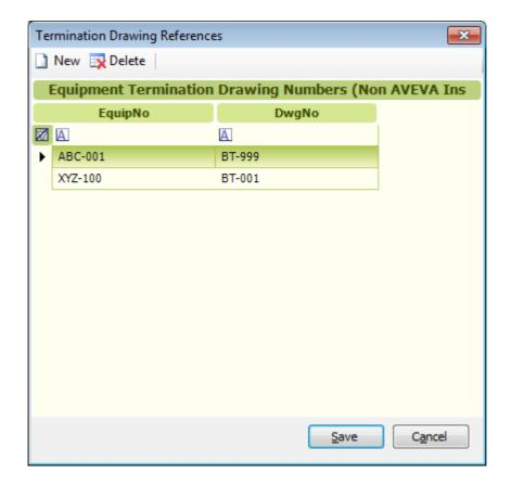
To add a new drawing reference, click **New**. A new row is then added to the window. Enter the equipment number and the drawing number in the fields provided.
