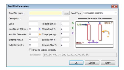
Complete all parameters as described, in the drawing units required in the AutoCAD drawing files (i.e. mm or inches)
