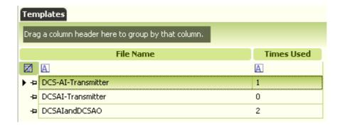
This window lists all the drawing files in the project template folder. **Times Used** shows the number of drawings in the Drawing list that use each template.
