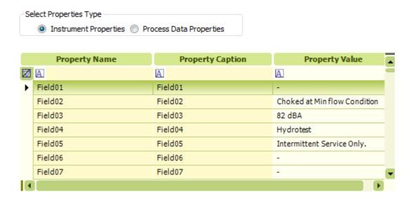
Use this tab to enter additional instrument and process data properties as required. Click on the appropriate **Select Properties Type** option and enter or edit values as required.
