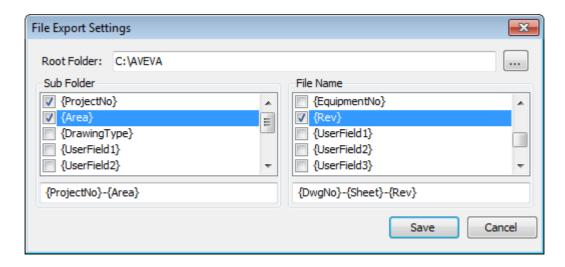
In the example above, a sub-folder structure of  $\{ProjectNo\}-Area\{Area\}$  and a file name format of  $\{DwgNo\}-\{Sheet\}-\{Rev\}$  have been selected. The selected root folder is "C:\AVEVA".
