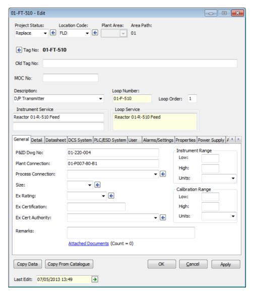
The two important fields for loop drawing generation are found on the Detail tab:
