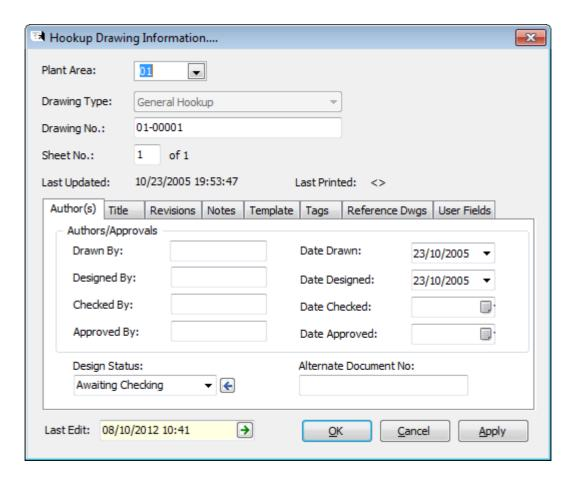
**Note:** The **Last Edit** field displays the date and time when the hookup drawing data was last edited. The user name of the individual that performed the edit is displayed in a tool-tip when the mouse cursor is hovered over the field. Click the button in the field to display the *Audit Manager*, which will display a list of all the changes to the hookup drawing data.
