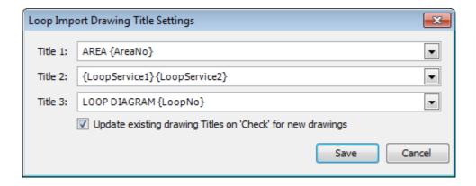
The window contains three fields that defines each of the Drawing List's title data fields. Each title can contain a mixture of text and DataLinks. On importing a new loop diagram from Engineer's Loop List, AVEVA Instrumentation will replace the DataLinks with the value for the database field within the DataLink. For example: Title 1 above is defined as: AREA {AreaNo}. When checking for new loops, if AVEVA Instrumentation found a new loop in area 21 then Title 1 would be: AREA 21.
