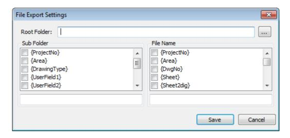
In the **Root Folder** field, enter the root folder under which the sub-folders that contain the exported files are to be located. Click the ... button to browse for the required folder.
