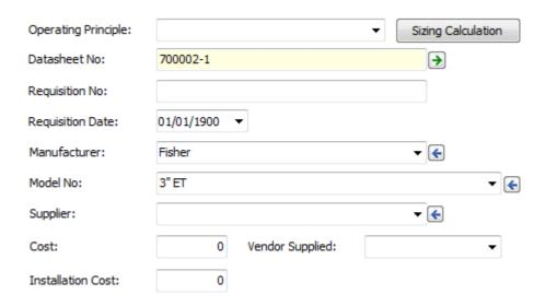
The **Operating Principle** PickList is used to pre-assign an instrument to a data sheet form type.
