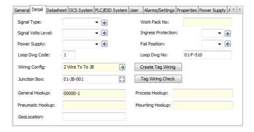
The Detail tab is used for more detailed design data and includes data typically required for wiring and installation information.
