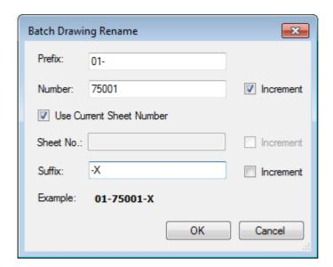
When the required fields have been completed the user must click **OK** to accept the values and display the **Select Drawings for Renaming** window or click **Cancel** to close the **Batch Drawing Rename** window and return to the grid view.
