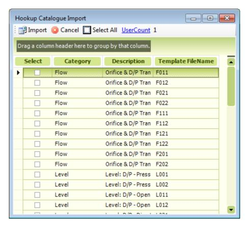
**Note:** To minimise the possibility that data currently being worked on by another user may be affected by an import, a list of the users working on the current project is available from the UserCount link. The number of current users is displayed next to the link. This total includes the user performing the import.
