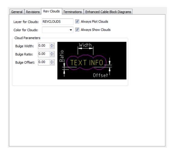
Changes to drawings are automatically highlighted using revision clouds if the **Cloud Changes** checkbox on the General tab (see above) is checked.
