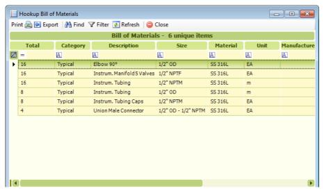
An item is added to the BOM by assigning it to a Hookup drawing and unchecking its **No.** checkbox (see *Assign Tags to a Hookup*).
