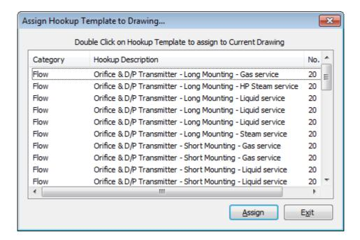
To assign a template either double-click on the Hookup Template record, or click on the Hookup Template record and then click **Assign**.
