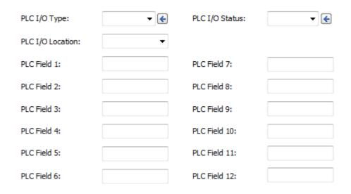
The PLC/ESD System tab is used to assign PLC or ESD (Emergency/Safety Shutdown) I/O information for the current tag (if the current tag will be connected to the PLC or ESD System).
