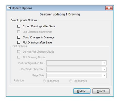
The window is used to specify whether or not the drawings are to exported when they are saved, whether or not changes in the drawing are to be highlighted with revision clouds, and whether or not the drawings are to be plotted when they are saved.
