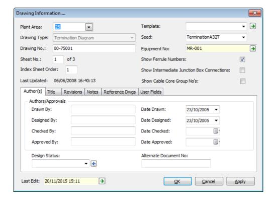
**Note:** All of the data entry fields in the **Drawing Information** window can be automatically updated for each drawing by using DataLinks to link the database data to drawing attributes.
