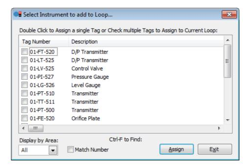
This window contains only those tags yet to be assigned to a loop. The tag list can be filtered to enable easy access to tags by area, using the **Display by Area** list.
