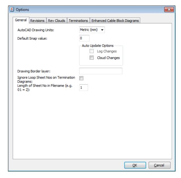
From the **AutoCAD Drawing Units** list, select Metric (mm) or Imperial (inch).
