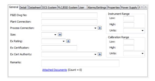
The General tab is used to enter typical common data for most instruments on the project.
