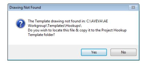
Click **Yes** to proceed. A window is then displayed which is used to browse for the required file. Once the required file is selected, click **Open** to open the drawing in AutoCAD and copy it to the Hookup template folder.
