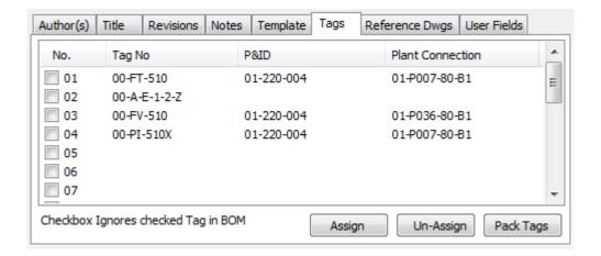
Drag the second tag and "drop" it onto the first position to move the selected tag to that position.
