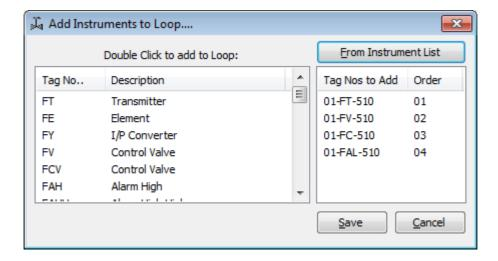
The left hand list shows typical tags and descriptions for the Engineer's ISA tag catalogue built using the current Loop function prefix in the **Edit Loop** window.
