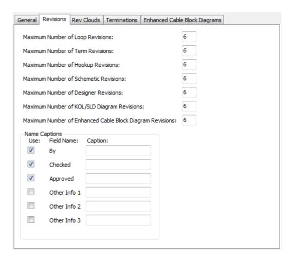
Enter the maximum numbers of loop, termination and hookup revisions that are to be listed on drawings in the fields provided.
