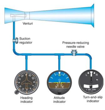
**Figure 3-27.** A venturi tube system that provides necessary vacuum to operate key instruments.
