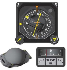
Figure 3-25. Pictorial Navigation Indicator (HSI Top), Slaving Control and Compensator Unit.
