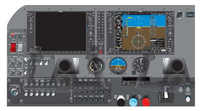
Figure 4-23. Reversionary Displays.
