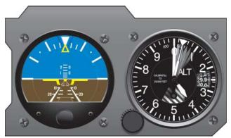
Figure 4-7. Pitch Correction Using the Altimeter.
