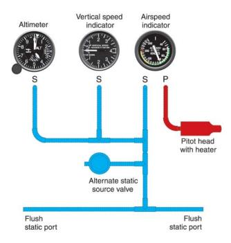
Figure 3-2. A Typical Pitot-Static System.
