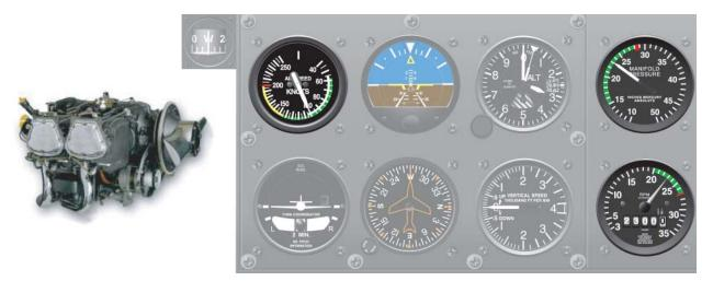
Figure 4-15. Power Instruments.
