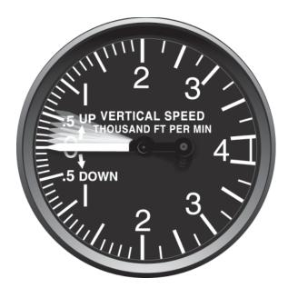
Figure 4-8. Vertical Speed Indicator.
