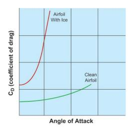
Ice on an airfoil can have other effects not depicted in these curves. Even before airfoil stall, there can be changes in the pressure over the airfoil that may affect a control surface at the trailing edge. Furthermore, on takeoff, approach, and landing, the wings of many aircraft are multi-element airfoils with three or more elements. Ice may affect the different elements in different ways. Ice may also affect the way in which the air streams interact over the elements.
