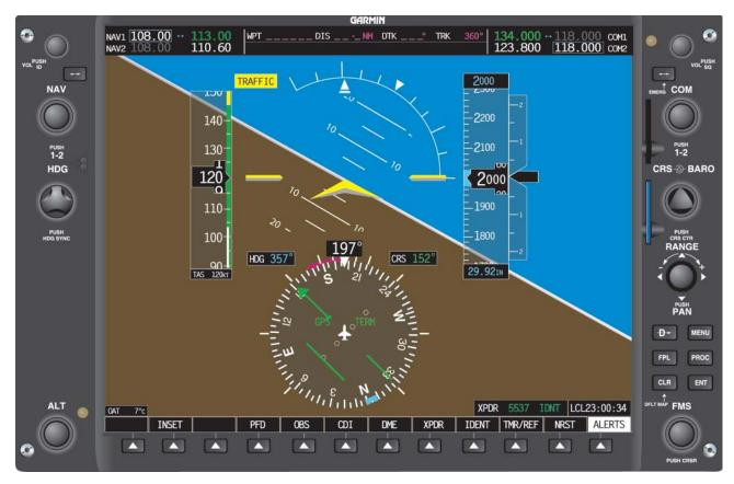
Figure 4-39. Horizontal Situation Indicator (HSI) Trend Indicator Elongates Proportionally With the Rate of Turn.
