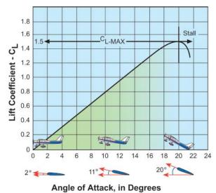
Figure 2-7. Relationship of Lift to Angle of Attack.
