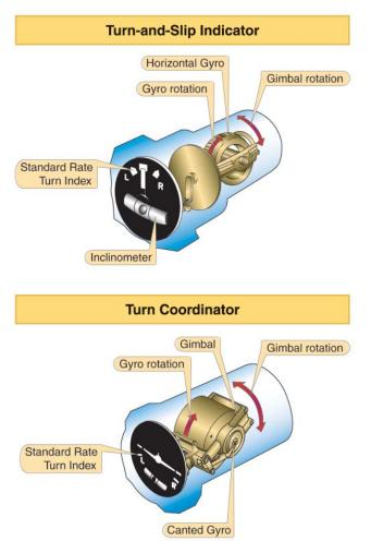
Figure 3-34. The rate gyro in both turn-and-slip indicator and turn coordinator.
