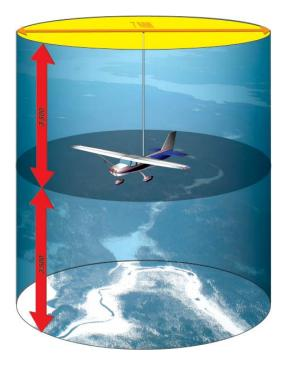
Figure 3-52. Coverage Provided by a Traffic Information System.
