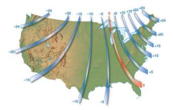
Figure 3-17. Isogonic lines are lines of equal variation.
