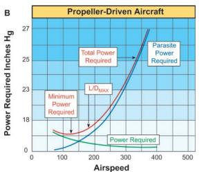
power setting can yield two speeds, points 1 and 2. This is because at point 1 there is high induced drag and low parasite drag, while at point 2 there is high parasite drag and low induced drag.
