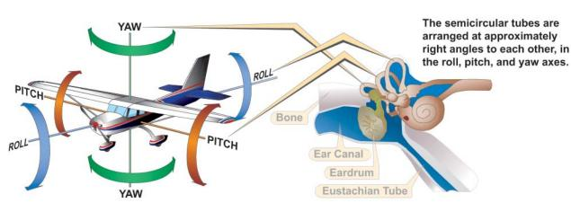
Figure 1-4. Angular Acceleration and the Semicircular Tubes.
