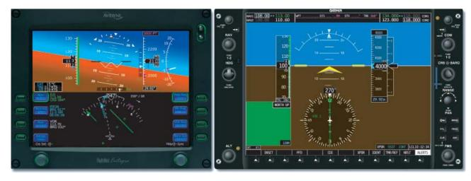
Figure 3-45. Two Primary Flight Displays (Avidyne on the Left and Garmin on the Right).
