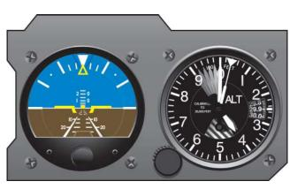
Figure 4-6. Pitch Correction Using the Attitude Indicator.
