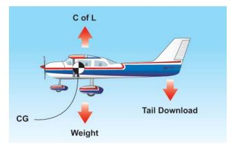
Figure 2-21. Downward Force on the Tailplane.
