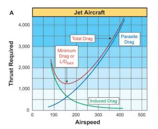
Figure 2-8. Thrust and Power Required Curves.
