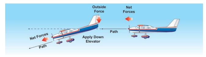
Figure 2-4. Newton's First Law of Motion: the Law of Inertia.
