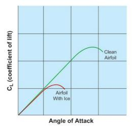
Figure 2-19. Aerodynamic Effects of Icing.
