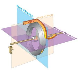
**Figure 3-32.** Precession causes a force applied to a spinning wheel to be felt  $90^{\circ}$  from the point of application in the direction of rotation.
