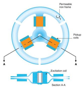
**Figure 3-23.** The soft iron frame of the flux valve accepts the flux from the Earth's magnetic field each time the current in the center coil reverses. This flux causes current to flow in the three pickup coils.
