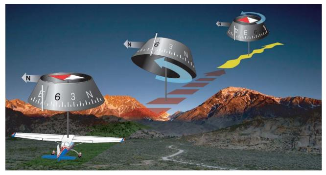
Figure 3-21. The Effects of Acceleration Error.
