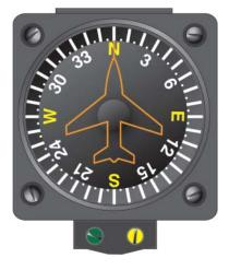
Figure 3-22. Vertical Card Magnetic Compass.
