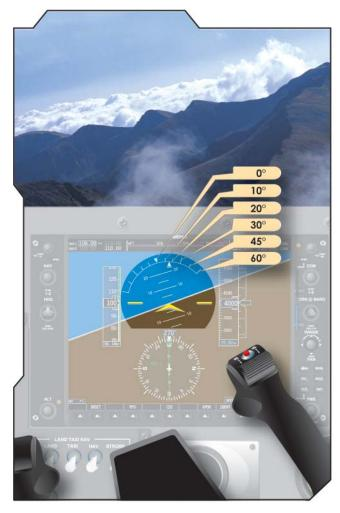
Figure 4-29. Bank Control Index Lines.
