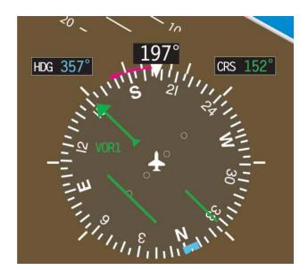
Figure 4-40. HSI Indicator (enlargement).
