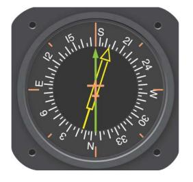
**Figure 3-26.** Driven by signals from a flux valve, the compass card in this RMI indicates the heading of the aircraft opposite the upper center index mark. The green pointer is driven by the ADF.
