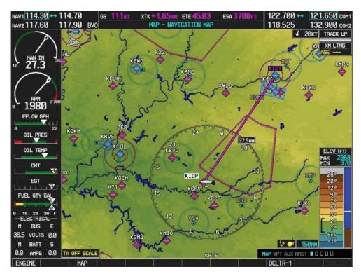
Figure 3-47. Example of a Multi-Function Display (MFD).
