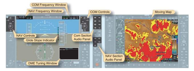
Figure 4-27. Navigation Instruments.
