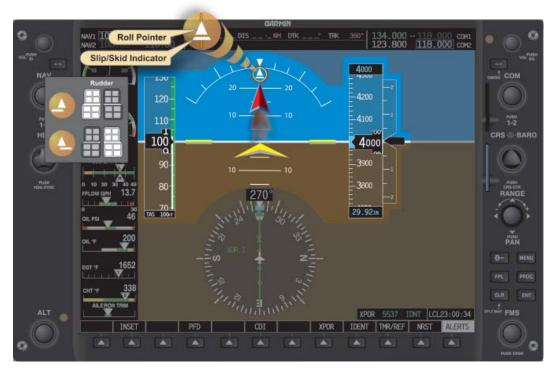
Figure 4-35. Roll Pointer and Slip/Skid Indicator.
