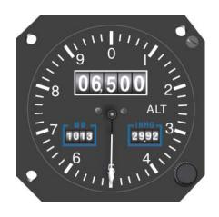
Figure 3-5. Drum-Type Altimeter.
