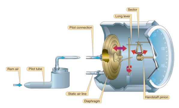
Figure 3-11. Mechanism of an Airspeed Indicator.
