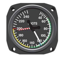
**Figure 3-14.** A maximum allowable airspeed indicator has a movable pointer that indicates the never-exceed speed, which changes with altitude to avoid the onset of transonic shock waves.
