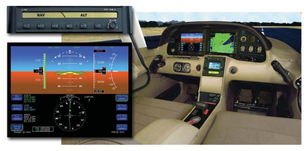
Figure 3-41. The S-TEC/Meggit Corporation Integrated Autopilot Installed in the Cirrus.
