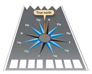
**Figure 3-18.** Utilization of a Compass Rose Aids Compensation for Deviation Errors.
