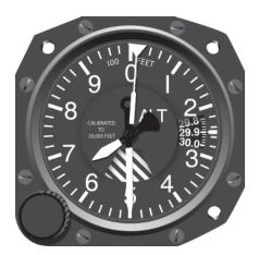
Figure 3-4. Three-Pointer Altimeter.
