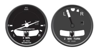
Figure 4-12. Turn Coordinator and Turn-and-Slip Indicator.
