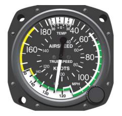
**Figure 3-12.** *A true airspeed indicator allows the pilot to correct IAS for nonstandard temperature and pressure.*
