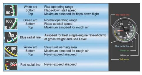
Figure 3-15. Color Codes for an Airspeed Indicator.
