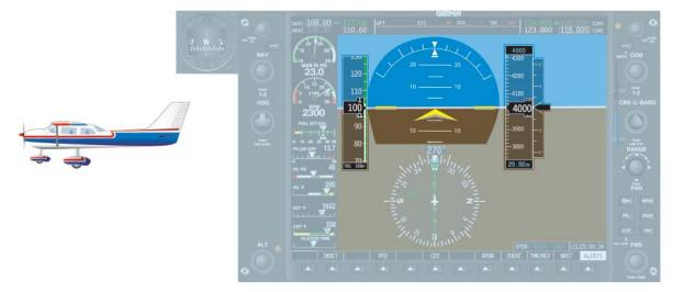
Figure 4-30. Pitch of the Aircraft.
