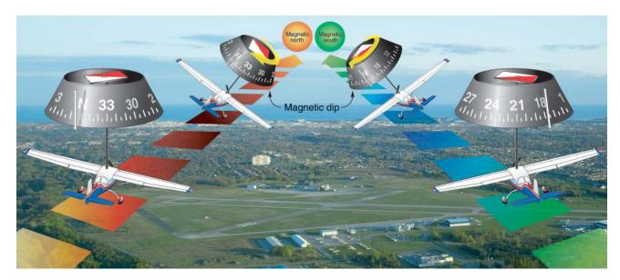
Figure 3-20. Northerly Turning Error.
