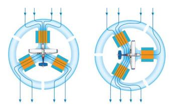
**Figure 3-24.** *The current in each of the three pickup coils changes with the heading of the aircraft.*
