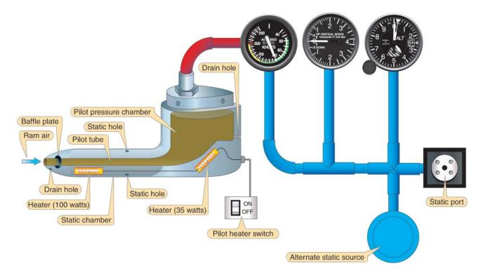
Figure 3-1. A Typical Electrically Heated Pitot-Static Head.
