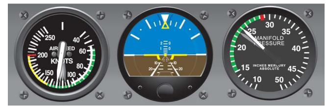
Figure 4-13. An Increase in Power Inscreasing Airpseed Accordingly in Level Flight.
