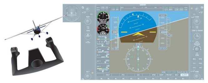
Figure 4-25. Control Instruments.
