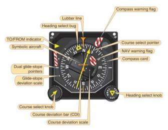
Figure 3-38. Horizontal Situation Indicator (HSI).
