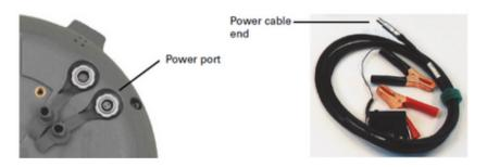
To connect the power cable, line up the red dot on the power cable end with the red dot on the power port and press into place. To disconnect the power cable, slide the cable collar (at the connector end) away from the unit and gently remove the cable.
