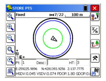
It is recommended that you face the front of the BRx5 head, so that your pole movements reflect the correct instrument orientation. But you do not need to look up. Look only at the level bubble indicator superimposed on the command. You will find that this speeds up field work dramatically and provides greater confidence in the accuracy of the GNSS measurements. A completely out-of-range for level computation would appear as shown below:
