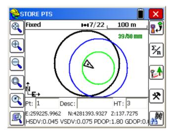
A perfectly centered bubble indicates perfectly level and would appear as shown here:
