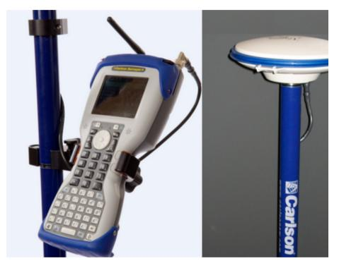
The Surveyor+ GPS system is specially designed for use as a rover with GNSS reference systems sich as Trimble VRS, Leica Spider, Topnet, Geodetics or Geo++. Communication is typically by cell modem. Note the two LED lights above the circular arrow key button, just below the screen. The LED on the right blinks steadily when corrections are being received.
