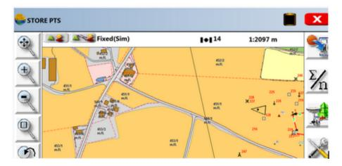
Shown below is SurvPC conducting snap-based stakeout (to screen elements) working native in a Microstation .dgn file:
