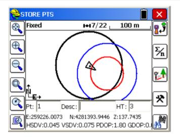
But when the tolerance is achieved, the inner circle becomes green. Then Enter or the icon for storing points can be pressed. If the tolerance is set to metric at 50 mm, then a calculation is made on the accuracy of the measurement, in this case 39 mm, within the tolerance setting.
