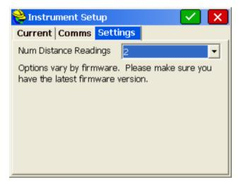
PTS3 instruments will first send out the last reading before sending the current reading. For some users, you may wish to choose to record the 3rd reading for the most accuracy.
