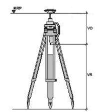
VO Vertical Offset VR Vertical Height Reading MRP Mechanical Reference Plane
