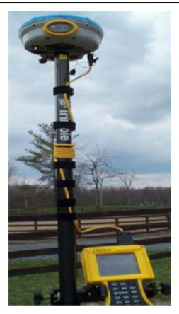
The Trimble 5800 with Zephyr antenna has a panel that includes an On-Off button at right.
