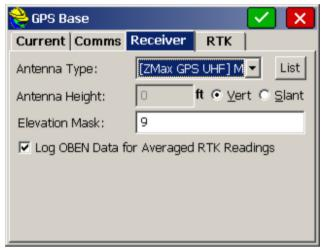
• Receiver tab - Antenna Type: A pull down list that includes approximately 50 different antenna types. Shown in the below photo is the Geodetic 4 antenna.
