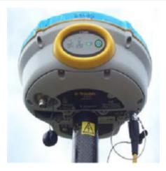
There are three LCD lights. From left, the first round light is yellow and flashes or pulses at 1 per second when sufficient satellites have been acquired for RTK, and flashes quickly when insufficient satellites are available. The second round light is a pulsing green light indicating radio linkage. When the pulse is intermittent, radio connection is being interrupted. The third, rectangular light is green and indicates battery status. It is steady on when there is sufficient battery power.
