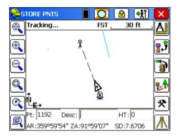
Next the icon has been toggled to non-tracking mode, which can be energy saving. No distances are taken in this mode.
