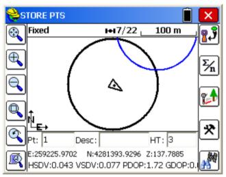
The LDL bubble indicator is turned on or off by checking the "Allow GPS Check Level" box in the View tab in the Configure section of Equipment as shown below:
