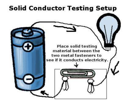
You can make a solid conductor testing set up with a battery, three wires, and a bulb as seen above. If a material is placed between the two metal fasteners that does conduct electricity, the bulb will light up. If the material placed between the fasteners does not conduct electricity, the bulb with not light up. In a way, by introducing a solid conductor into the circuit, and then removing it, you are creating a simple switch.
