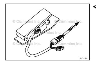
Remove the test lead from the last tested pin, insert it into the tachometer switch return pin. Measure the resistance from the tachometer switch return pin to the tachometer signal pin in the OEM harness connector.
