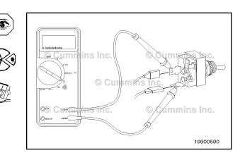
Move the switch to the OFF position and measure the resistance. The multimeter **must** show an open circuit (100k ohms or more). If the circuit is **not** open, the switch has failed.
