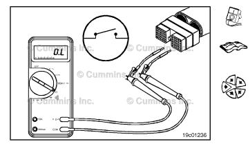
Remove the lead from the remote PTO switch return pin and insert it into the remote PTO switch signal pin of the harness connector. With the other test lead, check all other pins in the connector. Measure the resistance. The multimeter **must** show an open circuit (100k ohms or more).
