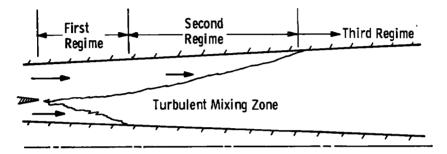
a. Mixing zone propagates to centerbody before it propagates to duct wall
