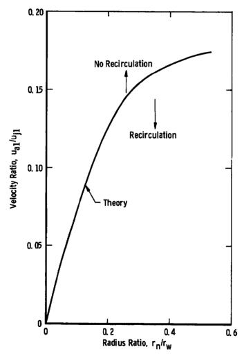
Figure 20. Limiting velocity ratio for recirculation in a constant-density flow within a cylindrical duct.
