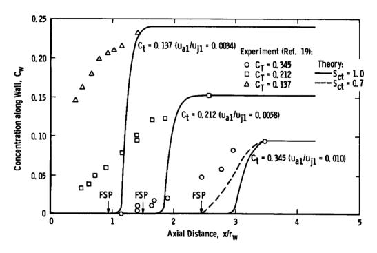
Figure 15. Wall concentration distribution for the experiments of Becker, et al.
