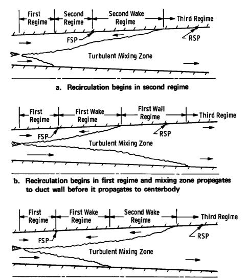
c. Recirculation begins in first regime and mixing zone propagates to centerbody before it propagates to duct wall
