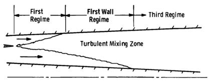
b. Mixing zone propagates to duct wall before it propagates to centerbody
