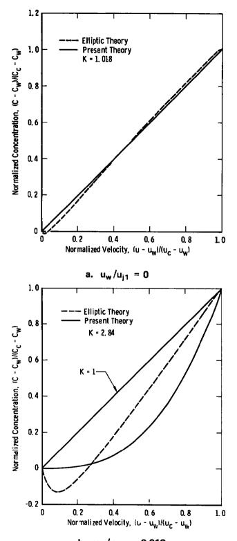
b.  $u_w/u_{j1} = -0.012$ Figure 19. Concentration-velocity relationship for the Barchilon and Curtet geometry,  $C_t = 0.305$ .
