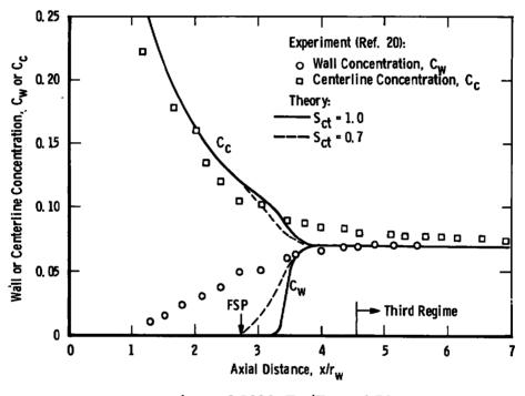
a.  $u_{a1}/u_{j1} = 0.0086$ ,  $T_{oj}/T_{oa} = 1.51$ Figure 16. Wall and centerline concentration distributions for  $u_{a1}$ .
