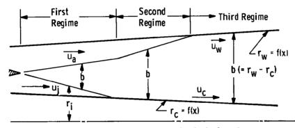
a. Mixing zone propagates to centerbody before it propagates to duct wall
