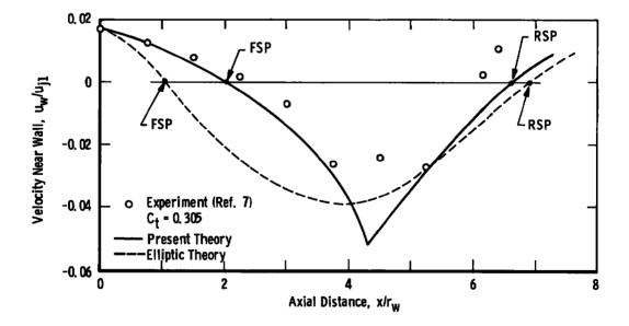
b. Velocity near wall Figure 18. Comparison of integral theory and elliptic theory for the Barchilon and Curtet geometry.
