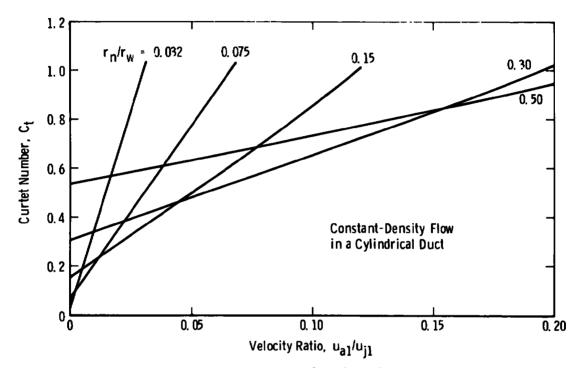
Figure 7. Curtet number as a function of velocity ratio.
