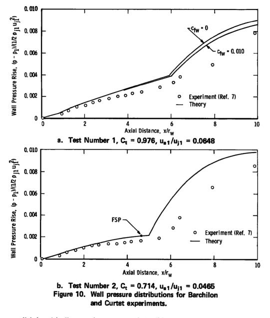
decrease slightly with distance downstream of the FSP, until a minimum is reached at a station upstream of the predicted shear layer attachment point.
