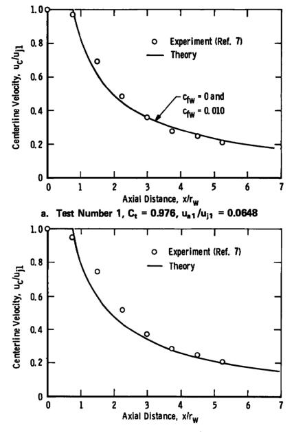
b. Test Number 2,  $C_t = 0.714$ ,  $u_{a1}/u_{j1} = 0.0465$ Figure 9. Centerline velocity distributions for Barchilon and Curtet experiments.
