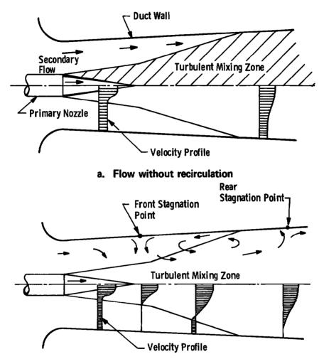
b. Flow with recirculation Figure 1. Schematic of ducted mixing processes.
