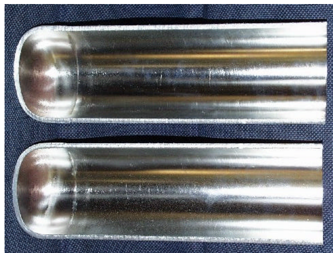
Figure 5-13 Photograph of the inside surfaces of a blind-holed 4-inch diameter pipe plated with nanocrystalline Co-P.
