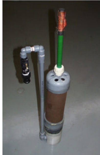
Figure 5-10 Photograph of the plating jig to plate the ID of schedule 40 (4” diameter) pipe.
