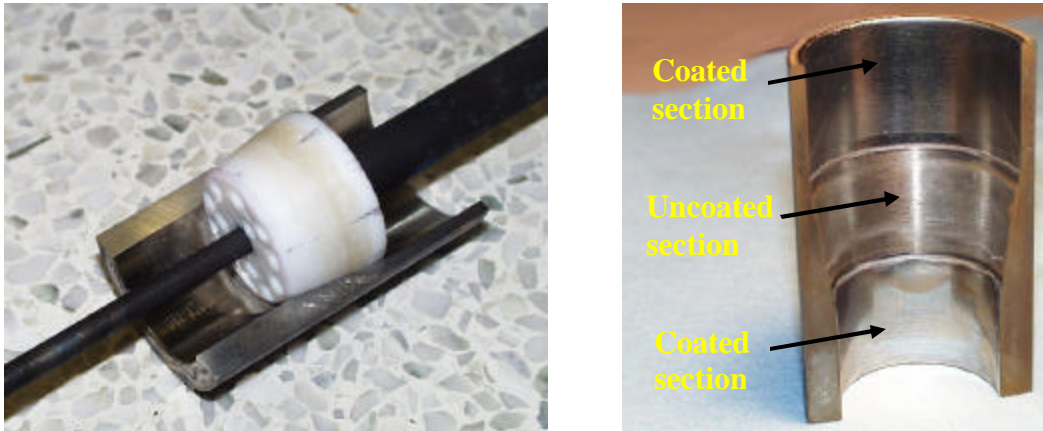
Figure 5-15 (a) Plated mock up sample ID3B (after sectioning) along with the plastic plug and the stepped graphite anode, (b) Photograph of the inside surface of a stepped ID (1.65/1.338inch) pipe showing coated and uncoated sections.
