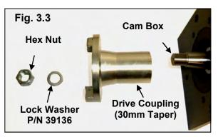
**Step 3** Position the mounting pedestal and connect the drive coupling to the test bench.
