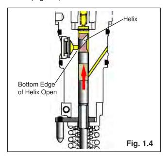
An engine driven governor, through linkage to the unit pumps, controls the rotational position of the pumping plunger. By turning the plunger different profiles on the helix will control the opening and closing of the charging port, tailoring timing and fuel delivery (Fig. 1.5).
