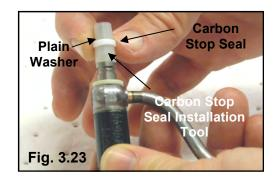
**Step 4** Allow the Carbon Stop Seal to relax for a few minutes. Then use the Carbon Stop Seal Re-sizing Tool in a slight rocking motion to squeeze the seal into its final size (Fig. 3.24).
