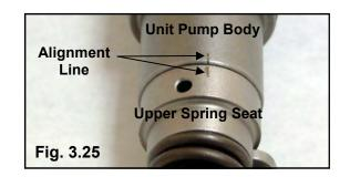
The stop positions are adjusted by changing the radial position of the Upper Spring Seat. This is accomplished by first adjusting the unit pump assembly in the cam box to a specified low idle fuel delivery. Then repositioning the upper spring seat to the full fuel rack position.
