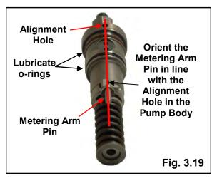
**Step 7** Install the unit pump into the Cam Box. Use the alignment hole as a reference to index the metering arm pin with the control rack slot (Fig. 3.19).
