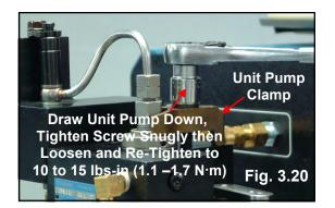
**Step 9** After seating the pump body in the cam box, loosen the hold down screw slightly and then tighten it to approximately 10 to 15 lbs-in (1.1 - 1.7N·m) as shown in Figure 3.21. This will provide a slight drag while rotating the unit pump during the clocking procedure.
