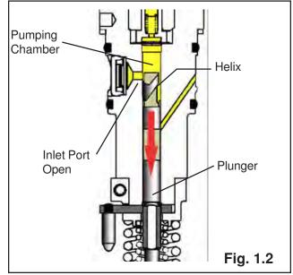
As the unit pump tappet is forced to rise due to the rotation of the engine driven cam, it causes the plunger to lift towards the pump body. The helix part of the plunger at a point defined by governor rack position closes off the inlet port. Fuel will no longer be spilled back through the inlet port; instead now it will be pumped at a much higher pressure to the injector (Fig. 1.3).
