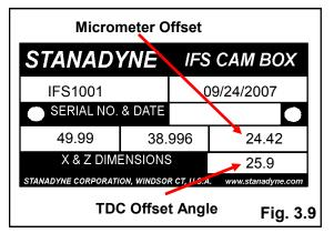
To verify the micrometer offset: Remove the o-ring seal from the micrometer adapter. Place the micrometer and adapter assembly on a flat surface, turn the micrometer in until it's spindle contacts the flat surface (Fig. 3.10). The reading should match the micrometer offset number stamped on the cam box nameplate (Fig. 3.9).
