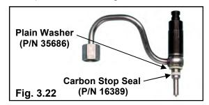
**Step 2** The CPN must be purged of air prior to system testing or the injection timing may be skewed during the test. To ensure that no air is entrapped within the injector, the CPN should be hydraulically locked using a suitable nozzle tester. Slowly increase the tester pressure until the nozzle opens, return to a pressure just below the nozzle opening pressure and maintain this pressure until the CPN is hydraulically locked (Reference Service Bulletin 557).
