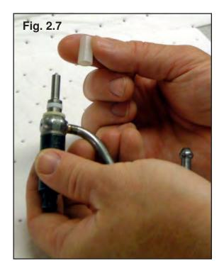
**Step 2** Place the carbon stop seal installation tool over the nozzle tip and slide the carbon stop seal over the 36528 installation tool (Reference Figures 2.6 and 2.7) until the seal drops into the groove on the nozzle holder body assembly. Remove and discard the installation tool.
