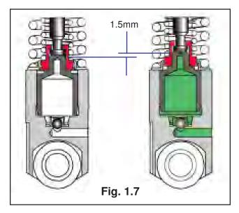
To meet today's and future emission standards, start of injection (SOI) to engine timing is critical. As previously explained, start of pumping that directly controls start of injection commences when the plunger rises in the pump body far enough that the pump plunger helix covers the inlet port.
