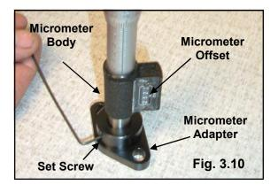
If the micrometer offset position is incorrect, the micrometer must be repositioned in the micrometer adapter as follows:
