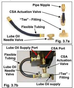
Before tightening the remaining fittings, determine a safe routing for the test bench's Lube Oil and Calibrating Oil tubing. Tighten the brass fittings securely in the cam box and connect the test bench hoses.
