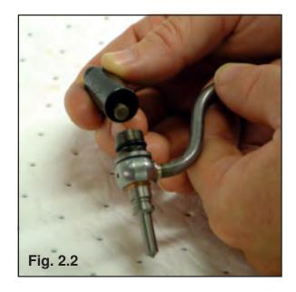
**Step 3** Apply a coating of clean calibrating fluid to the 35685 o-ring seal (Reference Figure 2.3) and hand tighten the cap nut onto the CPN body. Place the CPN in the 37745 holding fixture and using the 38021 CPN Cap Installation/Removal Tool tighten the cap to 110-120 lbf-·in (12.4-13.6 N•m) with a 3/4" (19mm) socket. Refer to Figure 2.3
