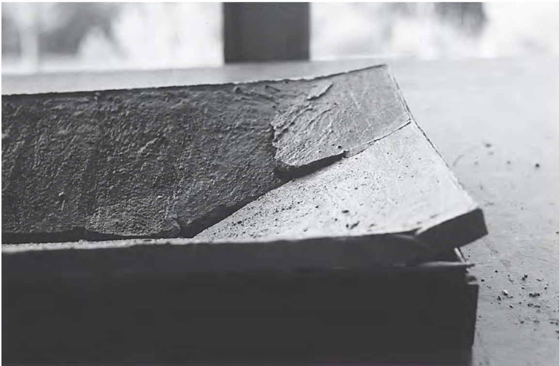
Figure 8: Corner crack of a simply supported beam under uniform transverse load. 10
