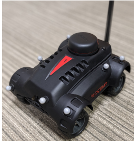
Fig. 2. The Ackermann-steered Hamster robot used in experiments. The markers are used to track the robot via an OptiTrack motion-capture system.
