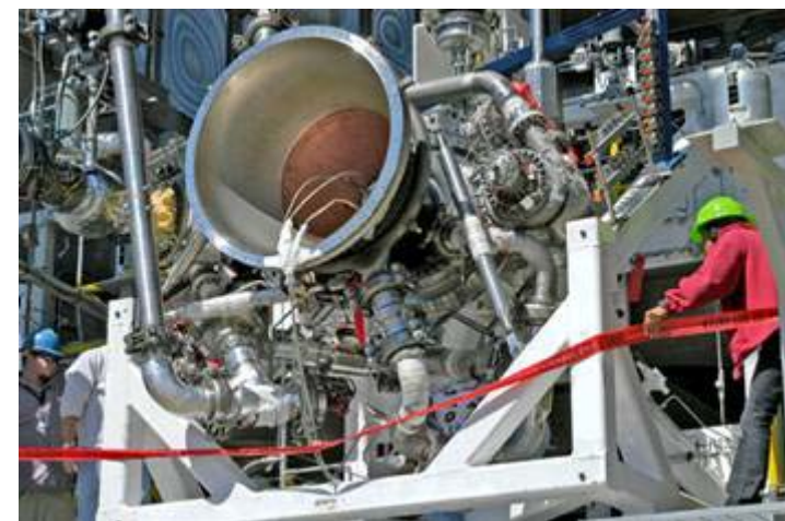
IPD Ground Demonstrator Engine installed in E1 Complex Cell 1
