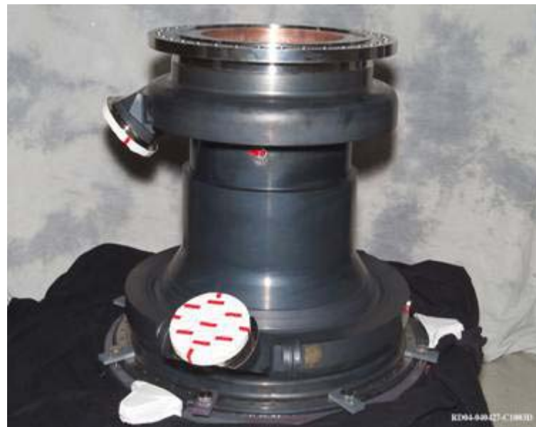
IPD HIP Bonded MCC (Boeing)
