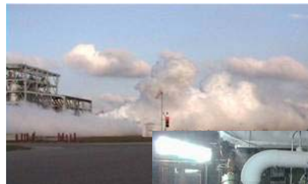
IPD Oxygen Pump in Hot Fire Testing
