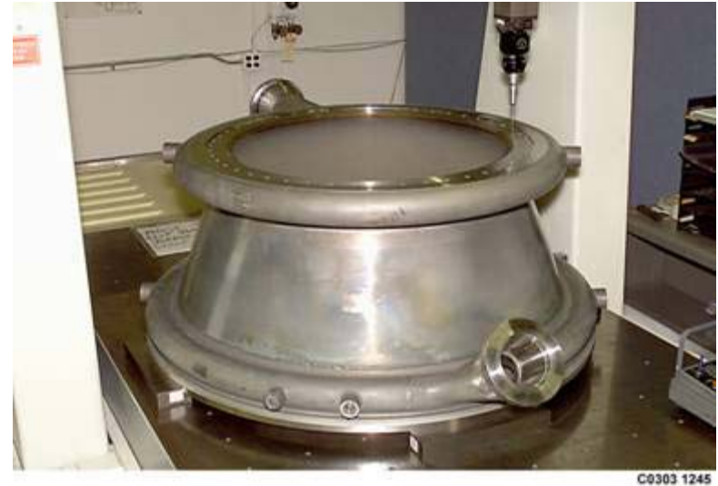
IPD Channel Wall Nozzle (Aerojet)
